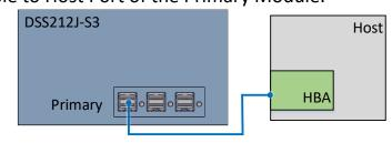
**Daisy-chain mode:** a single expander mode with expandable storage. The SAS HBA/RAID controller sees the collective HDDs from the daisy-chained DSS212J-S3s.
