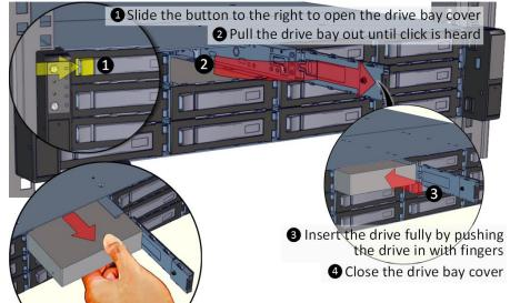
**To remove the disk,** open the drive bay cover, pull the handle out so that drive slightly slides out, and pull out the drive with hand.
