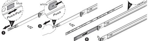
Ouretract the mid rail by pulling the latch on the mid rail
