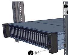
Install the fix mount rail to the rear posts
