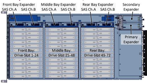
eDrawer4072J consists of three HDD backplanes. Every backplane has two internal expanders, each for SAS hard drive channel. See below diagram for board interconnection.
