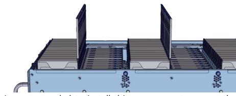
It is recommended to install drives per row, to ensure the easiness of inserting the tool-less trays back to their slots.
