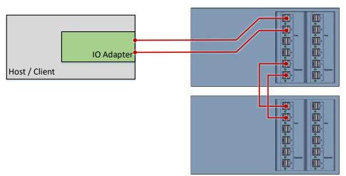
**Daisy-chain Configuration:** A single expander mode with expandable storage. The SAS HBA/RAID controller sees the collective HDDs from the daisy-chained eDrawer4072J units.
