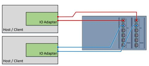
**Dual Expander / Clustered Storage Spaces Configuration:** SAS drives are required. In the above configuration, both hosts will have all the paths to all 72x disks at the same time.
