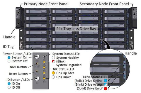
**3.** Install **3.5**" Drives to the unit as illustrated. It is suggested to install HDDs after the unit is mounted to the rack.
