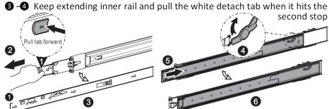
**5**–**6** Unretract the mid rail by pulling the latch on the mid rail
