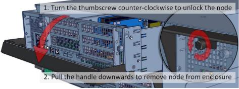
**5. Inspect the Controller Node**. The components comprise of a Tyan motherboard, an expander board, IO card, an NTB retimer board, NTB switch board, power board, 4x internal fan modules (all connected to the motherboard).
