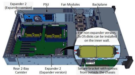
Using expanders, 12x SAS cables from backplane connect to 2x expanders, then from expander to SAS card (red path). For non-expander version, two 24-port SAS cards is required.
