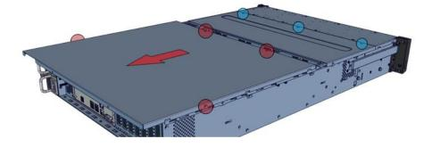
**4. Inspect the internal** of the chassis. FlacheSAN2V-D5 consists of a Tyan Purley motherboard, fan modules, backplanes, IO cards (optional) or expanders (for expander version) for 48x SSDs with internal mini-SAS HD cables.
