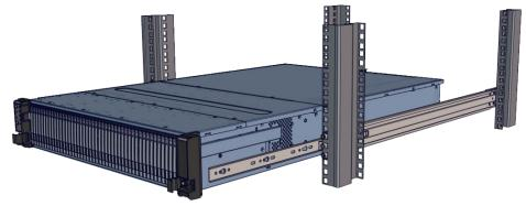
Refer to Rail Kit Installation Guide on complete detail on how to mount the unit. **Caution:** At least two people are required to lift a fully populated chassis
