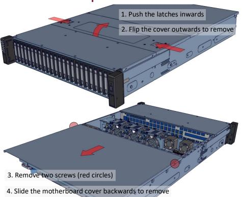
Remove the middle cover to get access to internal fans. The rear cover is for motherboard access.
