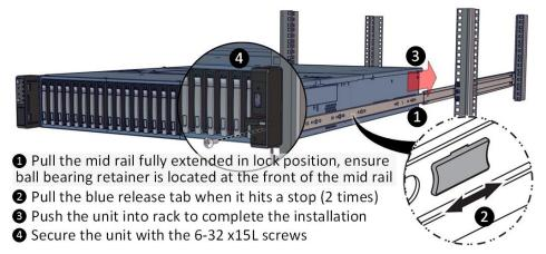
For a complete instruction on how to install unit to the rack, please follow the Slide Rail Installation Guide.
