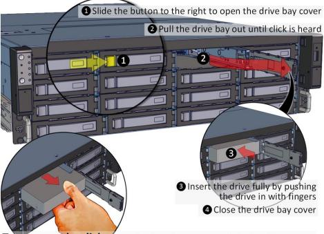
To remove the disk, open the drive bay cover, pull the handle out so that disk slightly slide out, and pull out the disk with hand.
