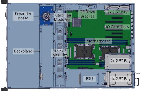
To install OS disk(s), a space for 2 OS disks is available on the left inner wall of the chassis.
