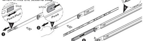
**5**–**6** Unretract the mid rail by pulling the latch on the mid rail
