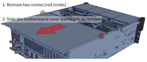
**4. Inspect the Inside** of the unit. Internal components comprise of a Tyan motherboard, an expander board, optional rear 2x and 8x 2.5" bays, 3x internal 120mm fan modules (electronically attached to the motherboard).
