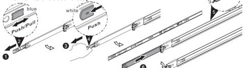
**9**–**6** Unretract the mid rail by pulling the latch on the mid rail
