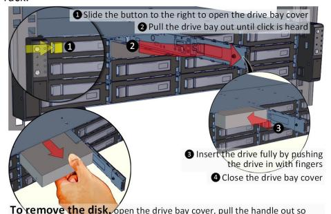
that drive slightly slides out, and pull out the drive with hand.
