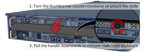
**5. Inspect the Controller Node**. The components comprise of a Tyan motherboard, an expander board, an NTB switch board, power board, 5x internal fan modules (all connected to the motherboard).
