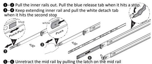
**10.** Install Inner Rails to the enclosure.
