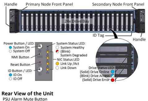
**3.** Install 2.5" Drives to the unit as illustrated. It is suggested to install HDDs after the unit is mounted to the rack.
