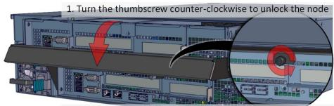
2. Pull the handle downwards to remove node from enclosure
