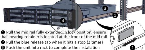
**4** Secure the unit with the 6-32 x15L screws
