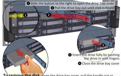
To remove the disk, open the drive bay cover, pull the handle out so that drive slightly slides out, and pull out the drive with hand.
