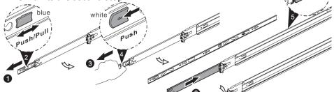
6 Unretract the mid rail by pulling the latch on the mid rail
