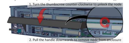
5. Inspect the Controller Node. The components comprise of a Tyan motherboard, an expander board, an NTB switch board, power board, 4x internal fan modules (all connected to the motherboard).
