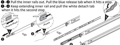
5–6 Unretract the mid rail by pulling the latch on the mid rail
