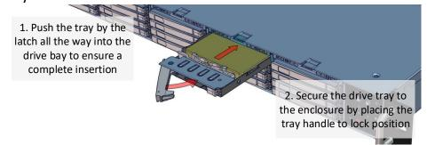
**13. Drive mapping** begins from top to bottom and to the right, depending on the internal SATA connection.
