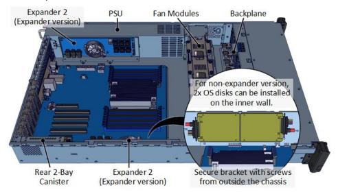
Using expanders, 12x SAS cables from backplane connect to 2x expanders, then from expander to SAS card (red path). For non-expander version, two 24-port SAS cards is required.
