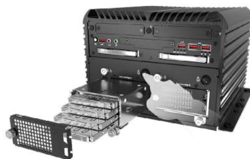
“Safety Eject” button for ensured safe hot swapping procedures
