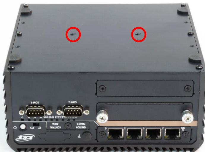
3. Place the din rail holder on top of the bottom cover and lock it with two screws (M4x5L, Nylok).
