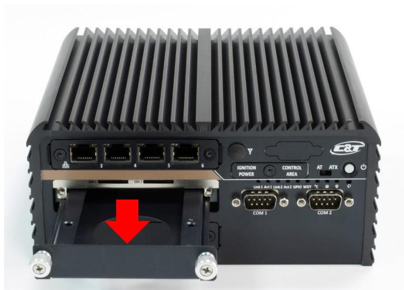
2. Lock the 2.5" HDD with HDD bracket using four screws (M3x4L).
