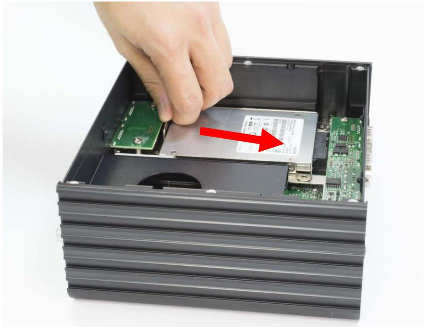
4. Fasten the four screws to lock the internal HDD bracket.
