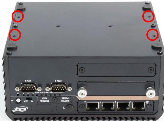
3. Lock the wall mount kit with eight screws (M3x5L, Nylok).
