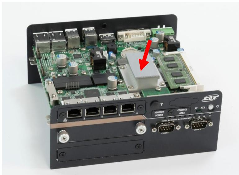
3. Hold the system body and slide the front/rear panel into the slide rail on the top cover.
