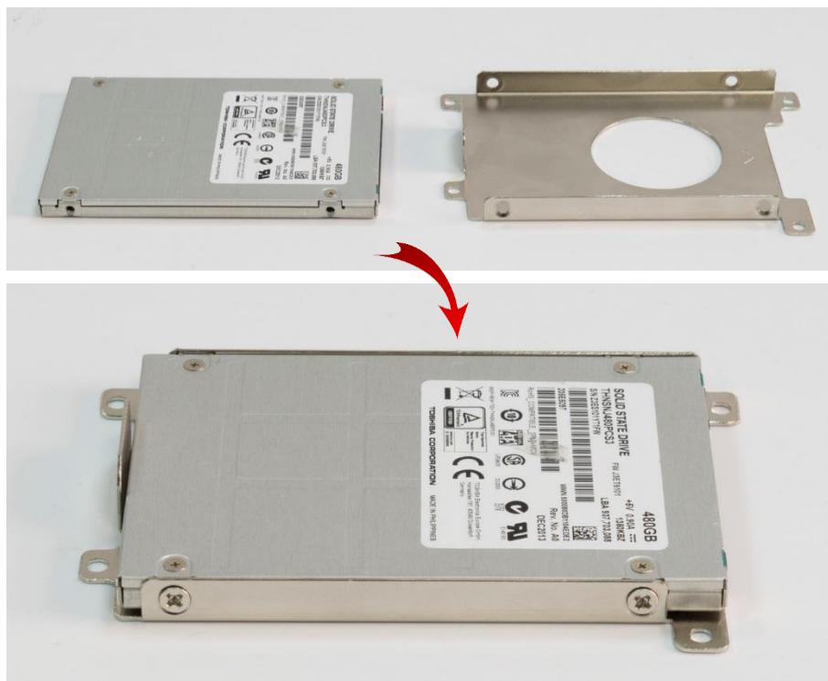
3. Install the HDD bracket following the direction below.
