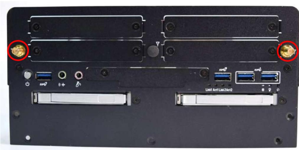
3. Assemble the antenna and SMA jack together.
