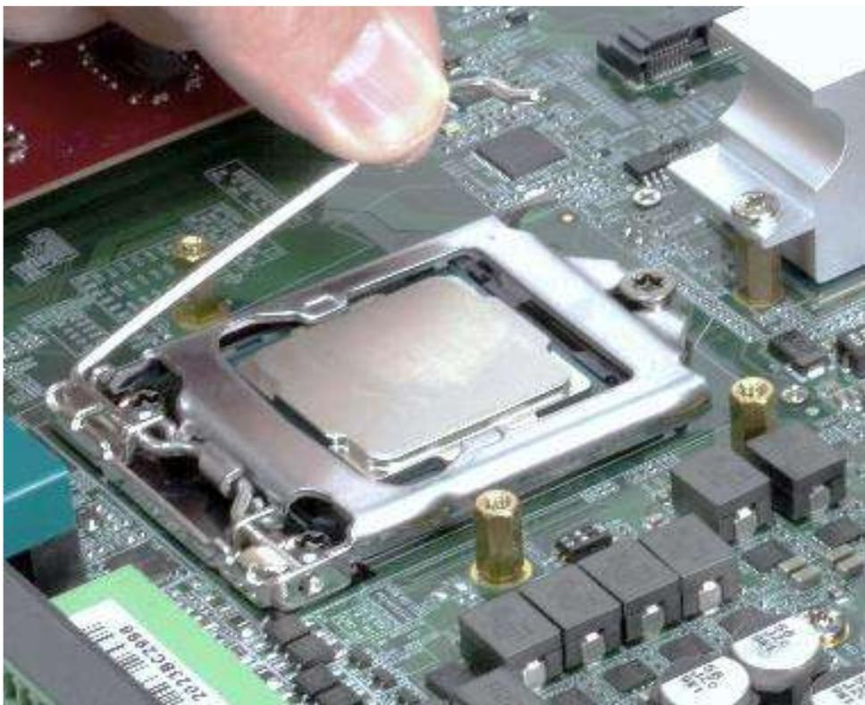
5. Paste thermal pad on the CPU.
