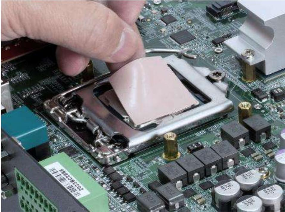
6. Place the designated heat block onto the CPU with thermal pad.
