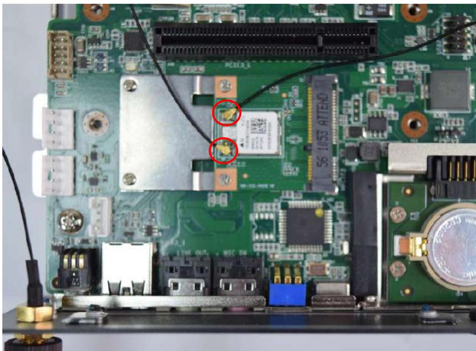
5. Assemble the antenna and SMA jack together.
