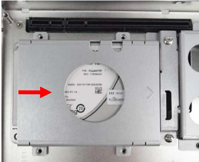
4. Fasten the 4 screws to lock the internal HDD/SSD bracket.
