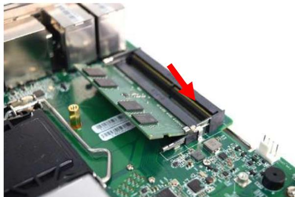
3. Press the memory module vertically downward until you hear the “click” sound. Make sure the memory module is firmly in place.
