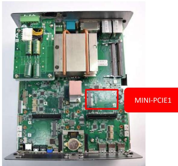
1. Insert Mini PCIe card from 45 degree direction.
