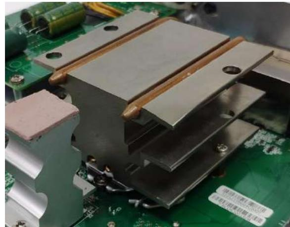
7. Lock the heat block with three screws (M3x8L). Screw driver will be able to penetrate through the holes on the top in order to fasten the screws with copper stud.
