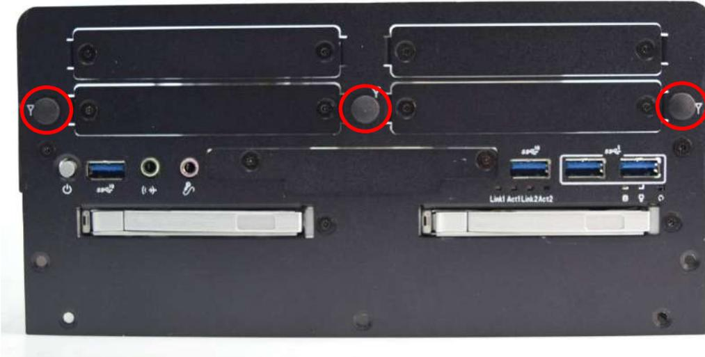
2. Have antenna jack penetrate through the hole, and fasten the nut with SMA jack
