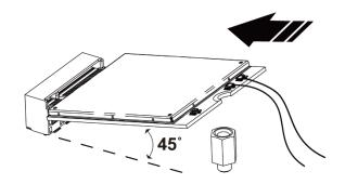
4. Press the communication module down and secure it with one screw.
