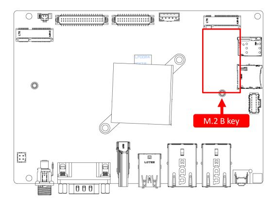
2. Connect the SMA cables to the communication (4G/LTE) module.
