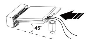
4. Press the Wi-Fi module down and secure it with one screw.
