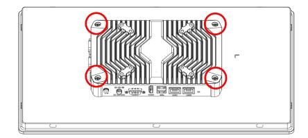
2. After removing the screws, detach the main unit from the screen.
