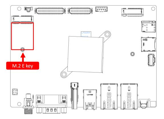
2. Connect the SMA cables to the Wi-Fi module.
