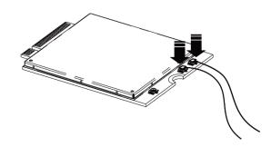
3. Insert the communication (4G/LTE) module at a 45-degree angle.
