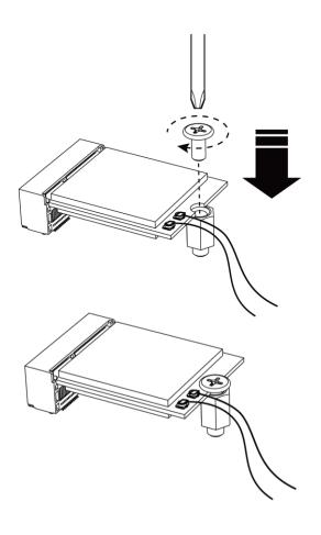
5. Ensure the internal antenna is securely connected to the network card, and the antenna interface is properly installed in the designated opening on the chassis cover.
