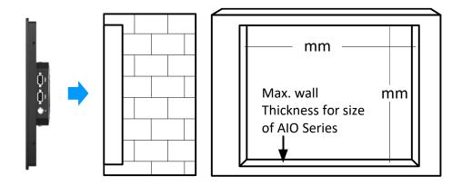
• From the FRONT of the wall, place the AIO Panel PC with its rear (display screen forward) into the measured cutout hole.
