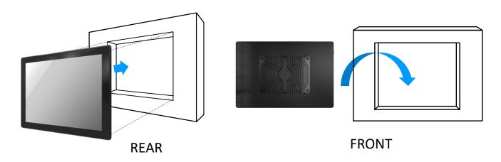
Install the mounting clips around the AIO and screw them in to secure against the wall. If the wall's thickness is greater than maximum wall thickness allowed, the clips will not fit. Please refer to the next page for the list of max wall depths
