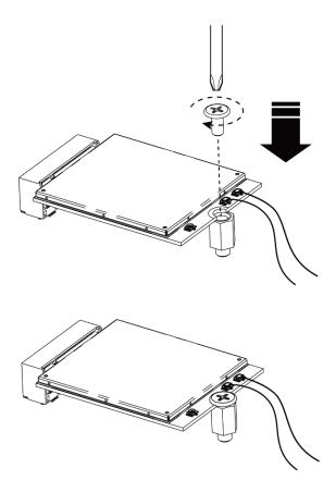
5. Ensure the internal antenna is securely connected to the network card, and the antenna interface is properly installed in the designated opening on the chassis cover.
