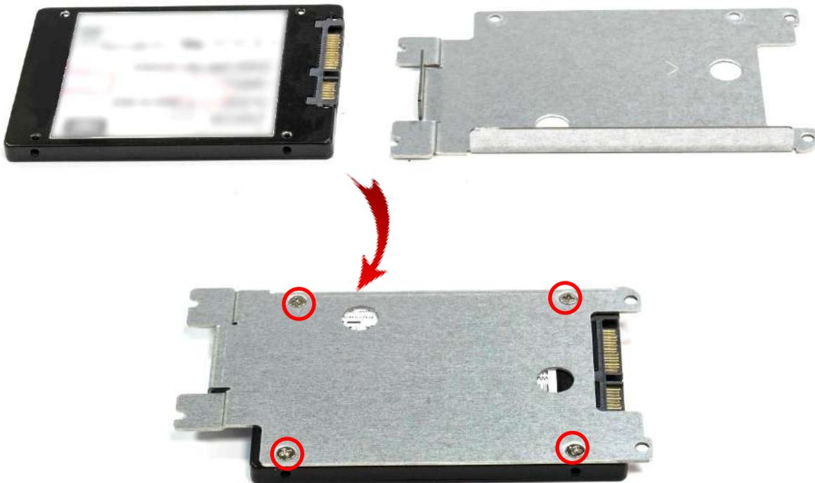
3. Insert the entire bracket following the below direction so the SATA connector is firmly plugged into the HDD.
