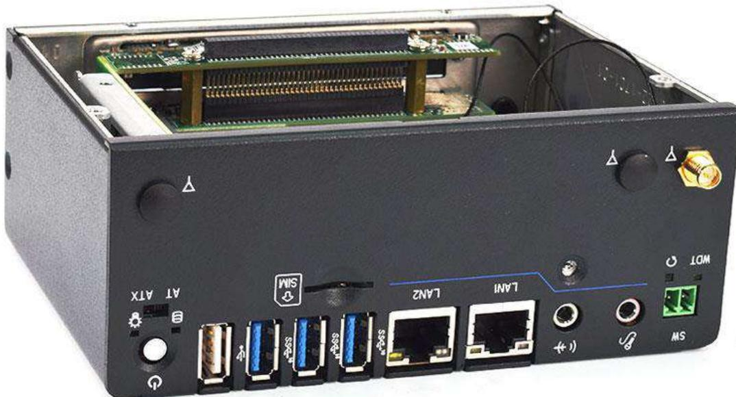
3. Put on washer and fasten the nut with antenna jack.
