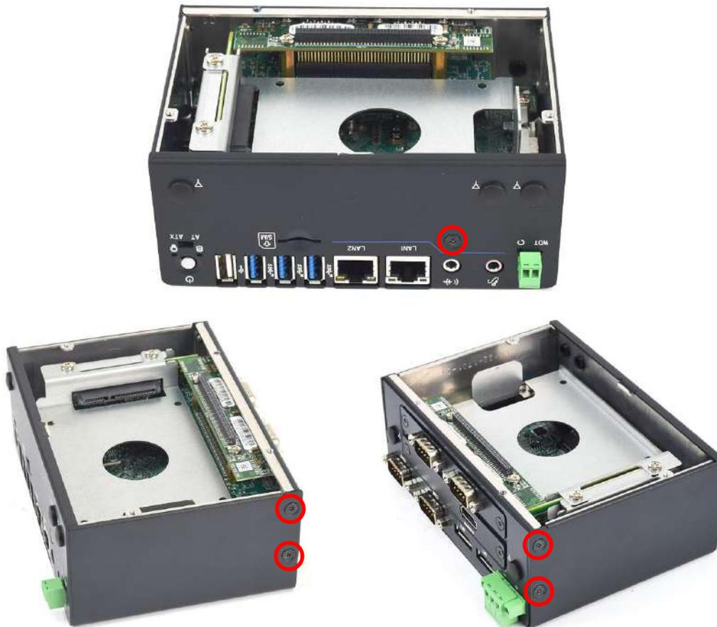
2. Hold the chassis top cover. Pull the system main body following the below direction so the top cover can be separated from it.
