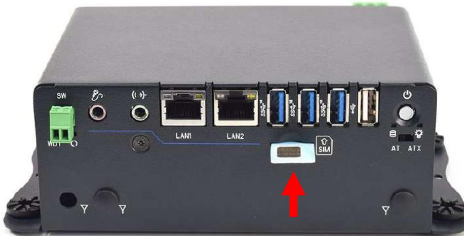
3. To uninstall SIM card, simply press the installed SIM card and then the card will be pushed out.
