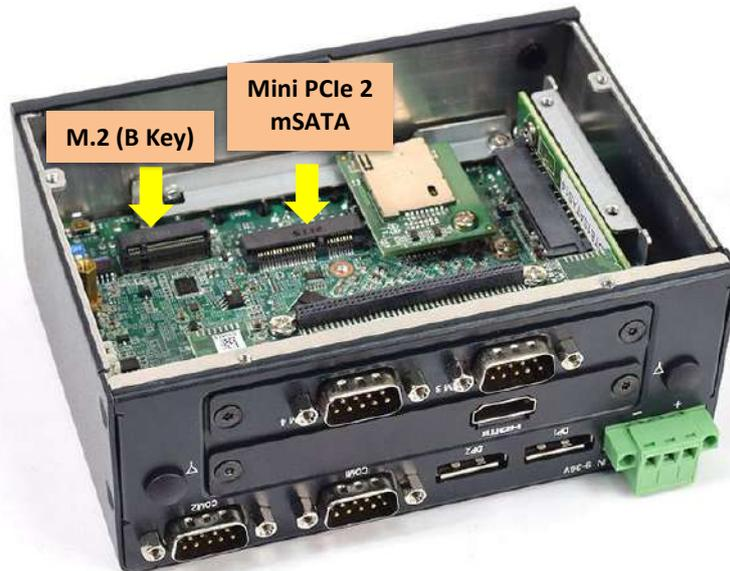
1. Insert mini PCIe card or mSATA module from 45 degree direction.
