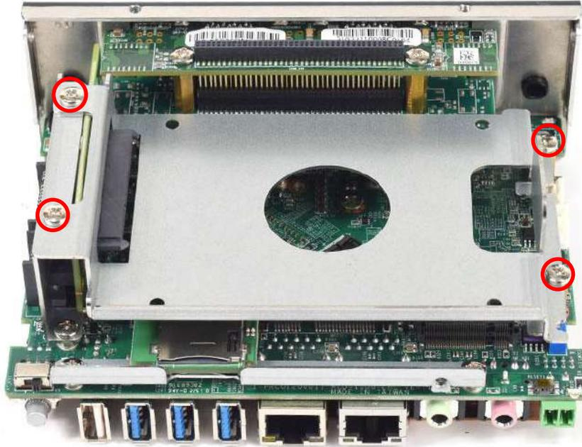
2. Lock the 2.5" HDD with HDD bracket using four screws.
