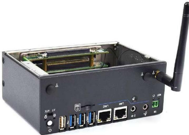
5. Attach the RF connector at the cable-end onto the communication module.
