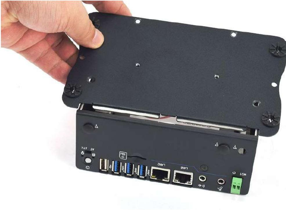
2. Lock the bottom cover with the four screws.
