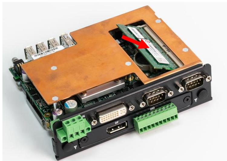
5. Press the memory module vertically downward until you hear the “click” sound. Make sure the memory module is firmly in place.
