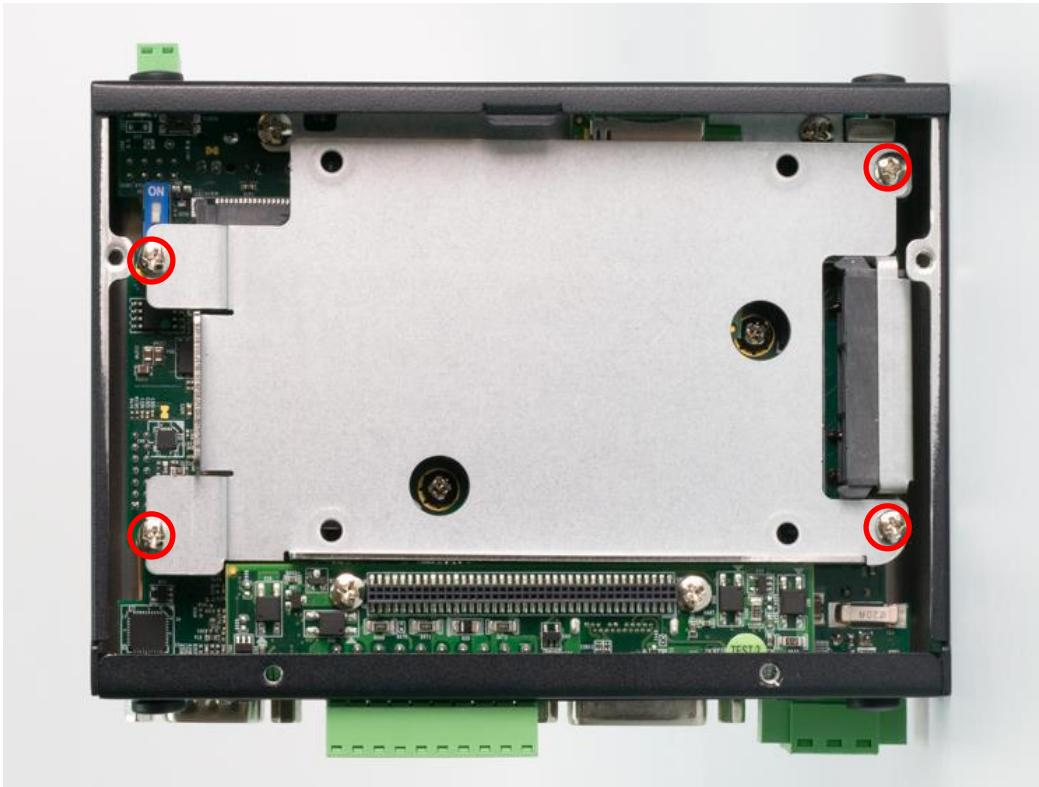
2. Lock the 2.5" HDD with HDD bracket using four screws.
