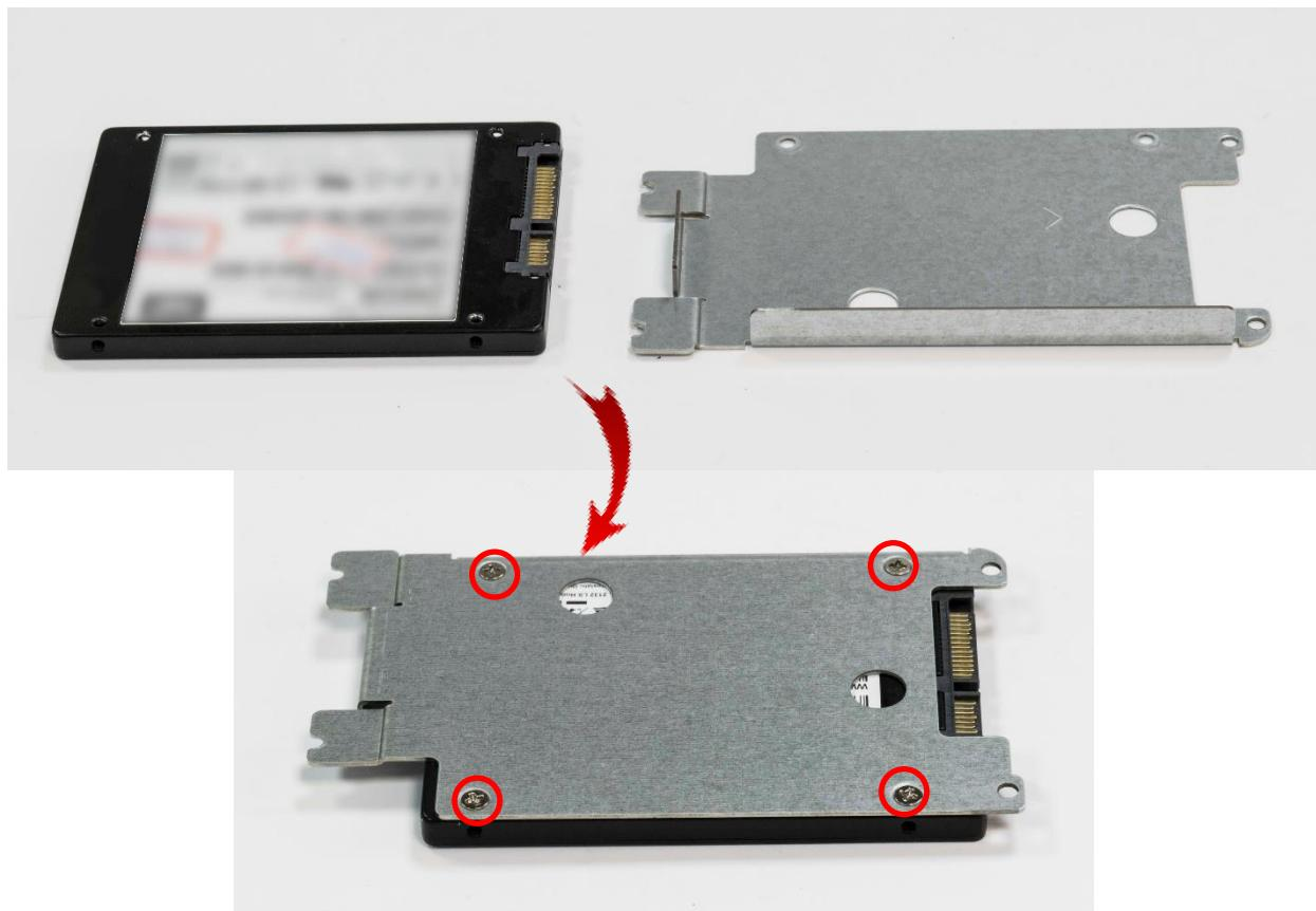
3. Insert the entire bracket following the below direction so the SATA connector is firmly plugged into the HDD.
