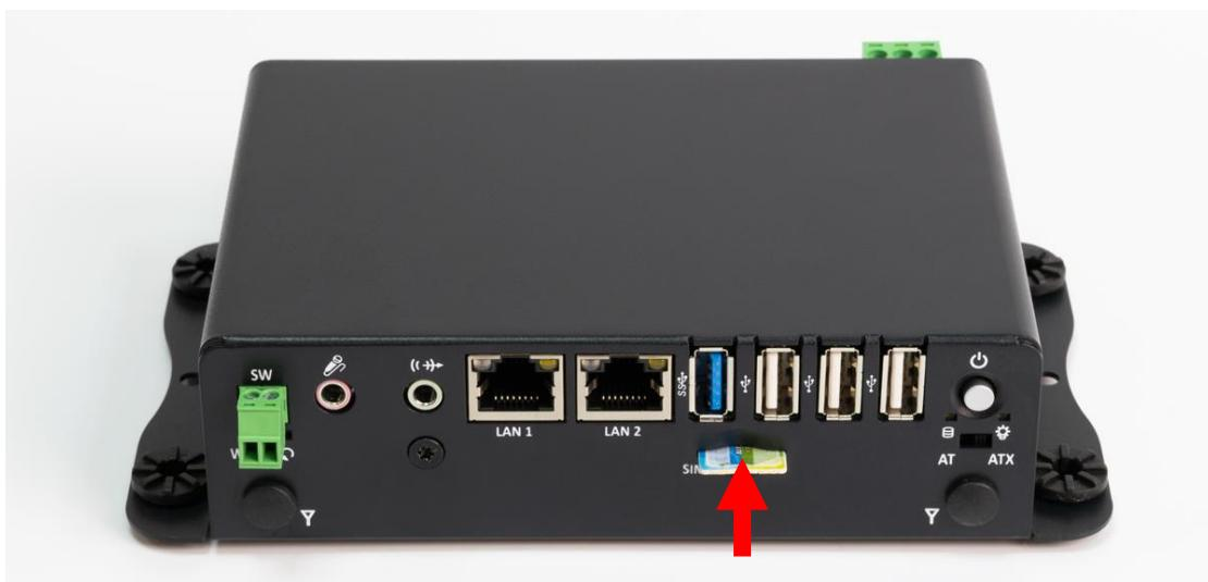
3. To uninstall SIM card, simply press the installed SIM card and then the card will be pushed out.
