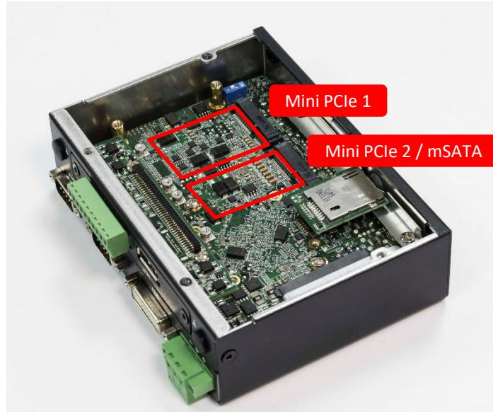
2. Insert mini PCIe card or mSATA module from 45 degree direction.
