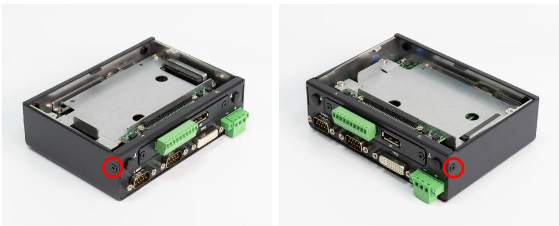
2. Hold the chassis top cover. Pull the system main body following the below direction so the top cover can be separated from it.
