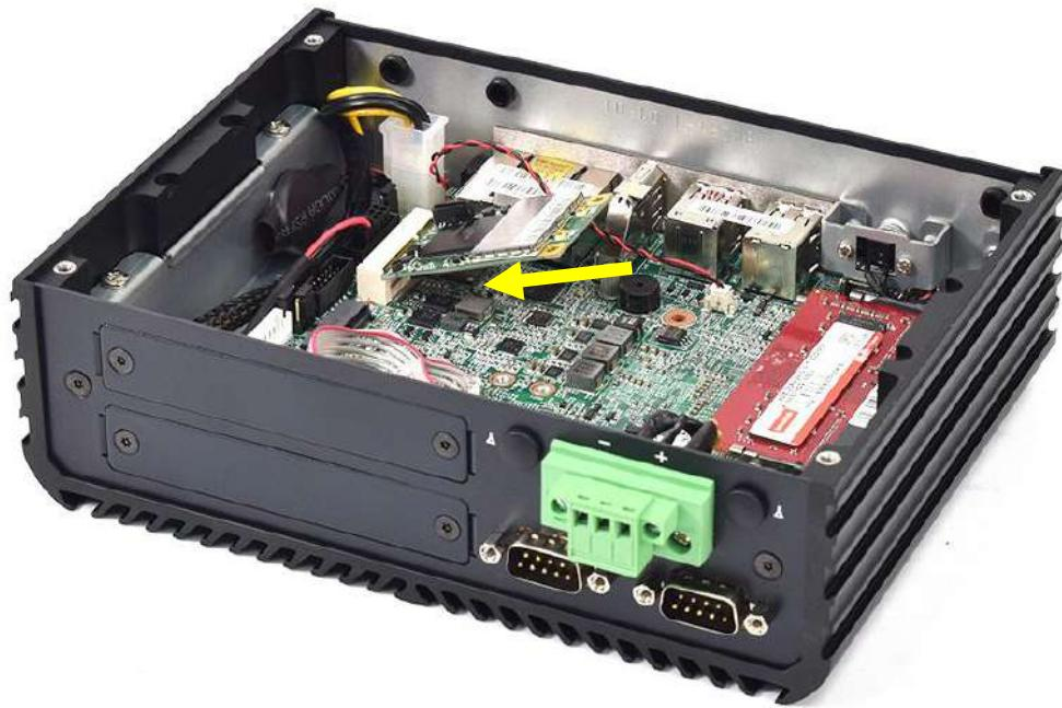
2. Press the mini PCIe card or mSATA module down and lock it with one screws (M2.5x5L).
