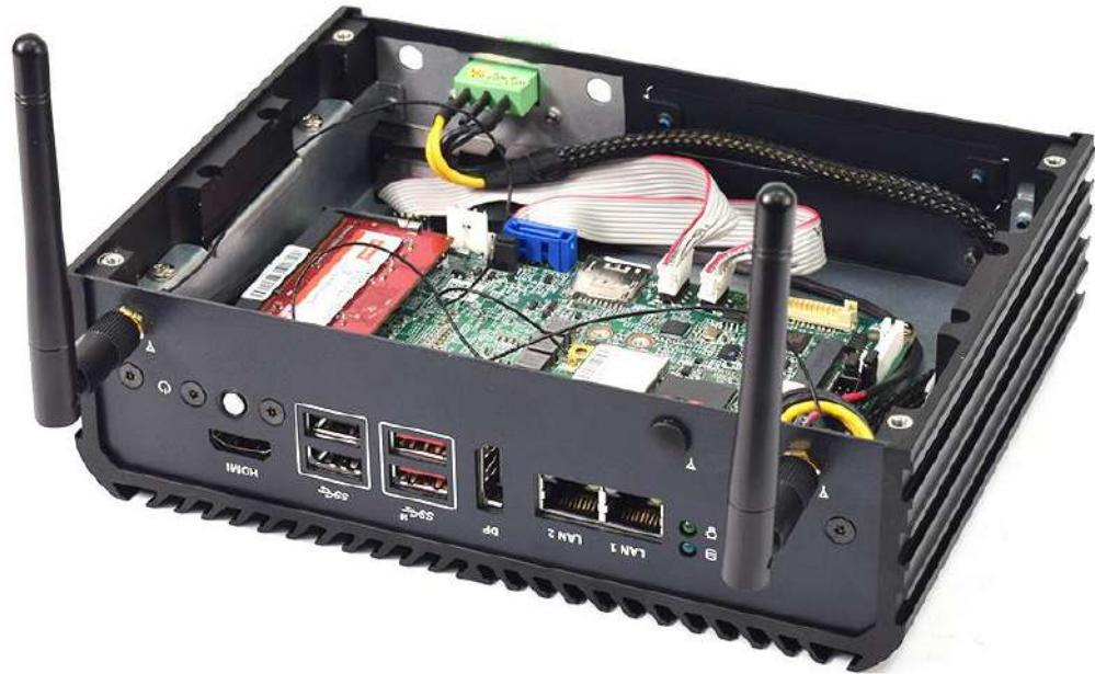
**5. Attach the RF connector at the cable-end onto the communication module.**
