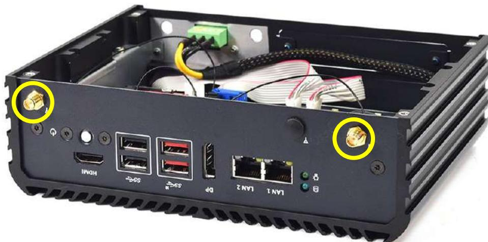
3. Put on washer and fasten the nut with antenna jack.
