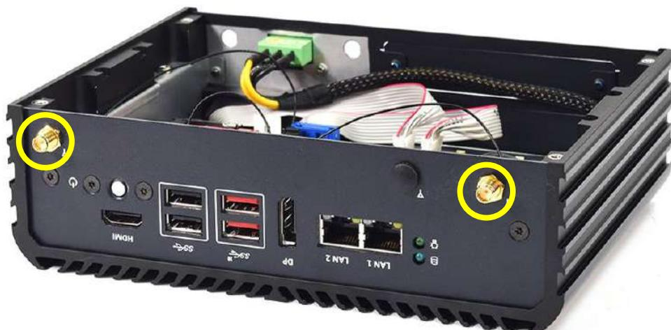
**4. Assemble the antenna and antenna jack together.**
