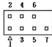
**JDIO1: GPIO Connector (8 bits)**
