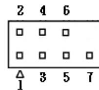
**JDIO1: GPIO Connector (8 bits)**
