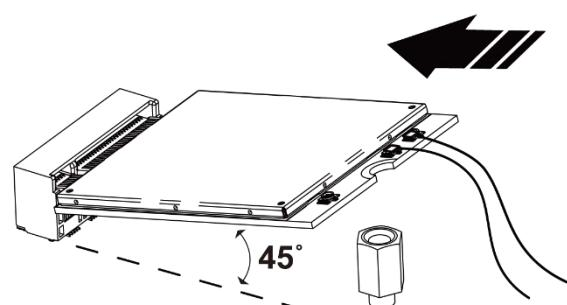
4. Press the communication module down and secure it with one screw.
