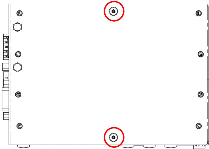
2. Remove the four screws on the left side of the computer.
