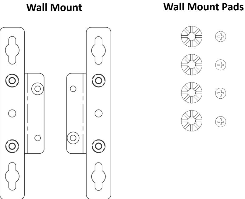
2. Assemble the anti-vibration grommets and screws together.
