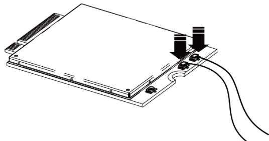
3. Insert the communication (4G/5G) module at a 45-degree angle.
