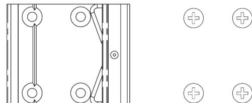
2. Place Din rail holder on the back of computer and secure it with four screws.
