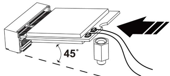
4. Press the Wi-Fi module down and secure it with one screw.
