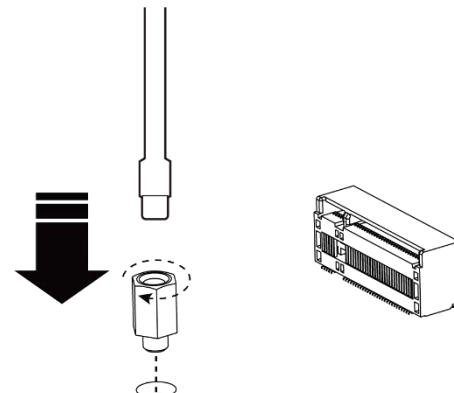
2. Insert the NVMe SSD at a 45-degree angle into the M.2 B-Key slot.
