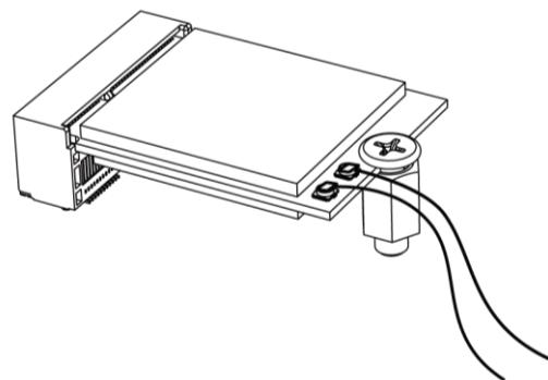
6. Attach the external antenna to the SMA jack by securely threading them together.
