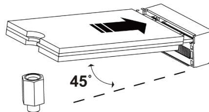
3. Press the NVMe SSD down and secure it with one screw.
