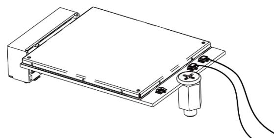
5. Assemble the antenna and SMA jack together; the outcome should resemble the picture below.
