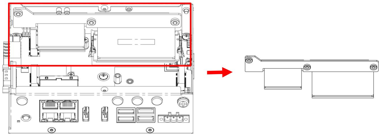
2. The M.2 B Key slot supports NVMe SSD, as highlighted in the picture below.
