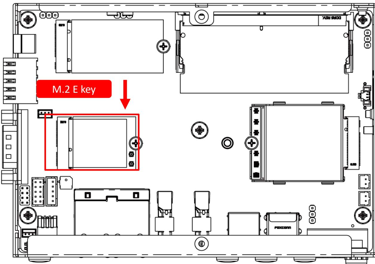
2. Connect the SMA cables to the Wi-Fi module.
