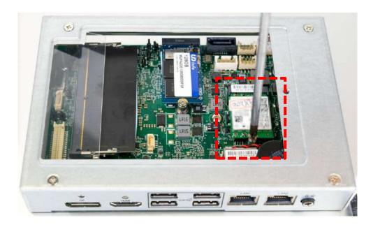
2. Route the antenna cable out of the main unit and attach the antenna to a non-metallic surface away from the whole body. (Do not attach it on iron parts)
