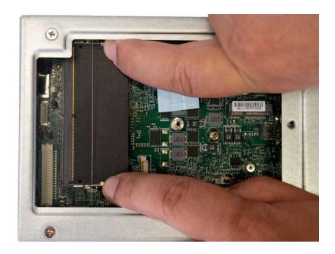
2. After the memory module pops up, pull it out. Carefully remove the thermal pad underneath the memory module.
