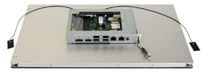
3. If it is necessary to attach the antenna to the main unit, ensure that at least half of the antenna's surface area is exposed and extends beyond any iron parts.
