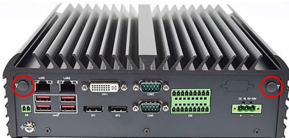
4. Have antenna jack penetrate through the hole, and fasten the nut with SMA jack.
