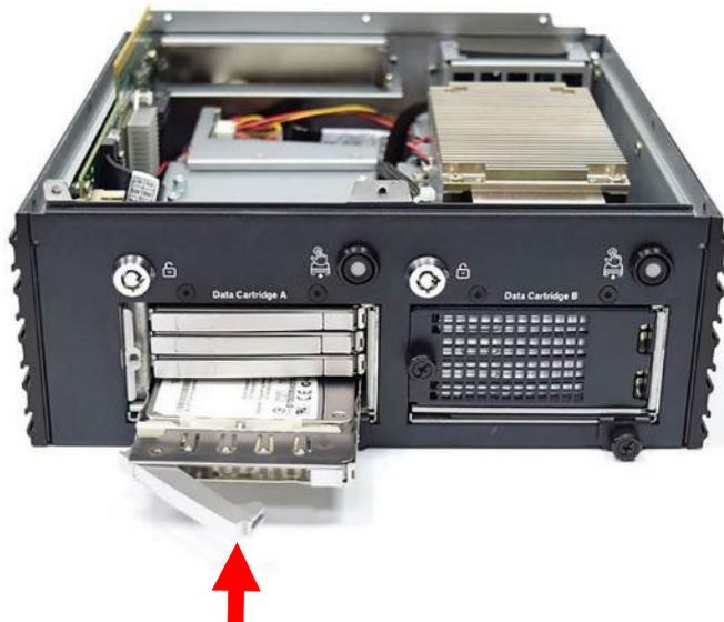
**5. Unscrew the toolless screw circled below to take out the NVMe canister**
