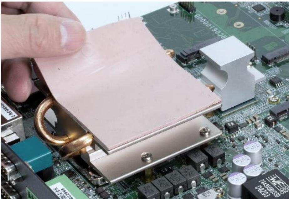
**9. Paste the thermal pad onto the installed heat block.**
