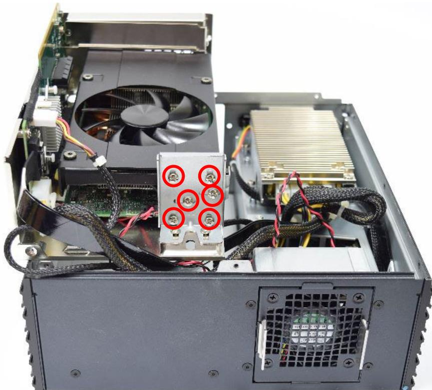
**6. Fasten the 2 screws and Insert power cable from the power board to the graphic card.**
