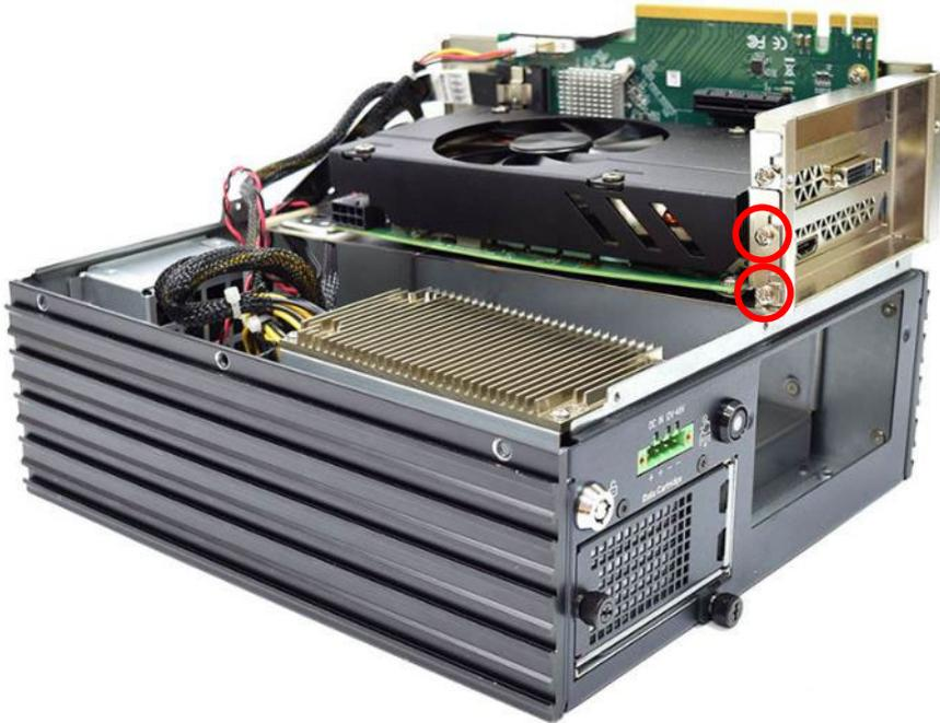
5. Adjust the arm until it holds the card firmly in place. Then fasten the screw on the holder.
