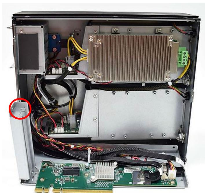
4. Install the PCIe/PCI extension card and ensure the gold finger is inserted into the slot. and then fasten the screw.
