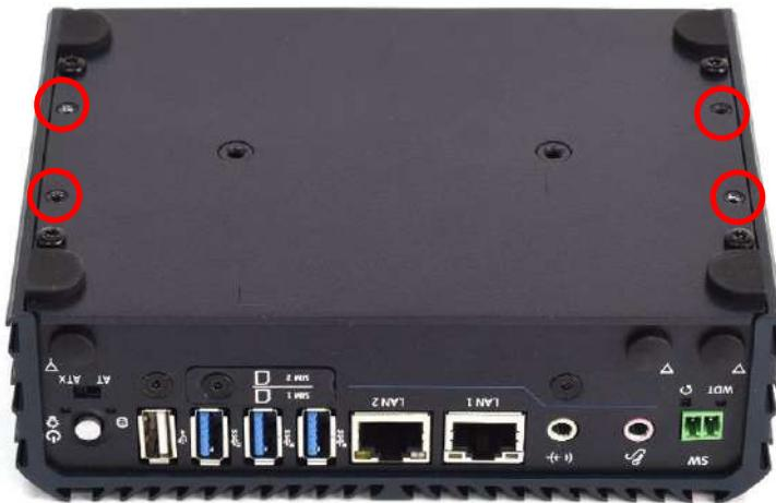
3. Place the VESA mount kit (for system) on top of the system aligning the matching screw holes.
