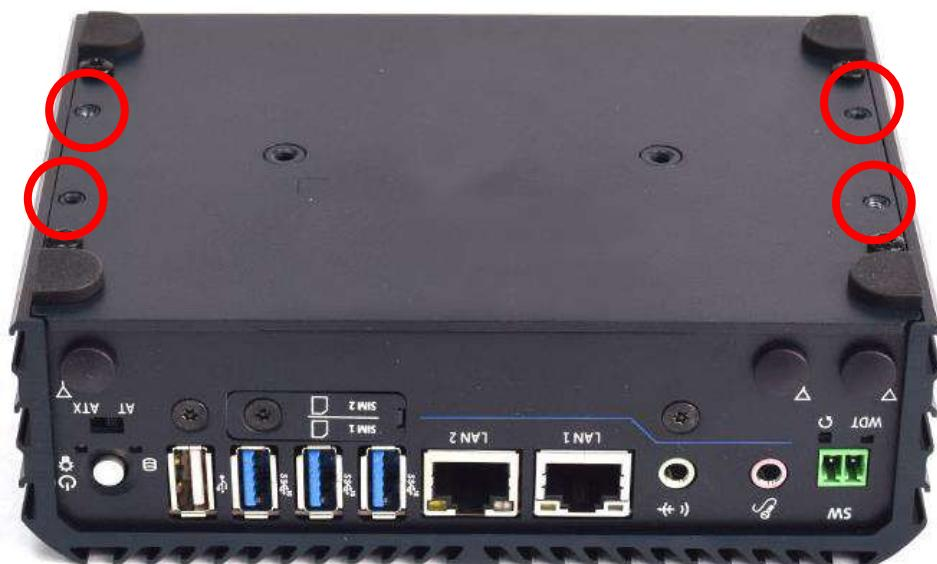
3. Lock the wall mount kit with eight screws (M3x5L, Nylok).
