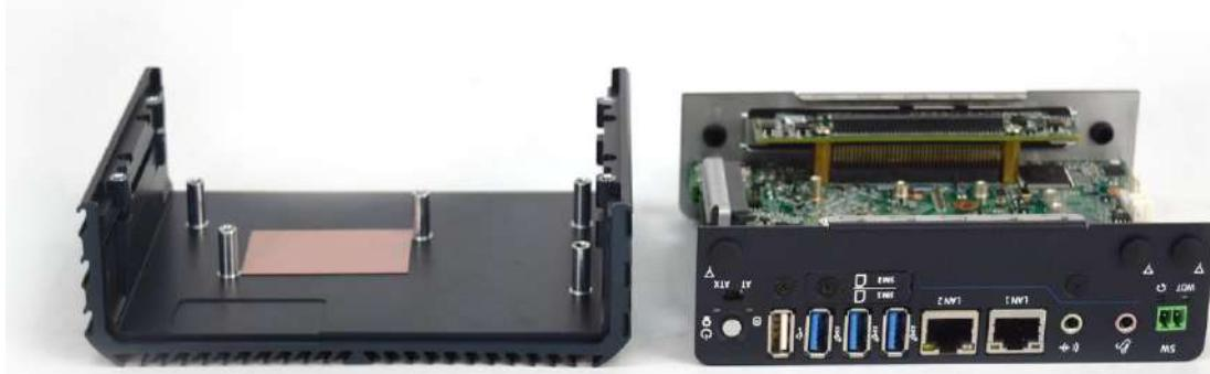
2. Ensure thermal pad is in place where the CPU is located or paste the thermal pad back on the CPU thermal block.
