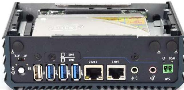
3. Press the entire bracket following the below direction so the SATA connector is firmly plugged into the HDD.
