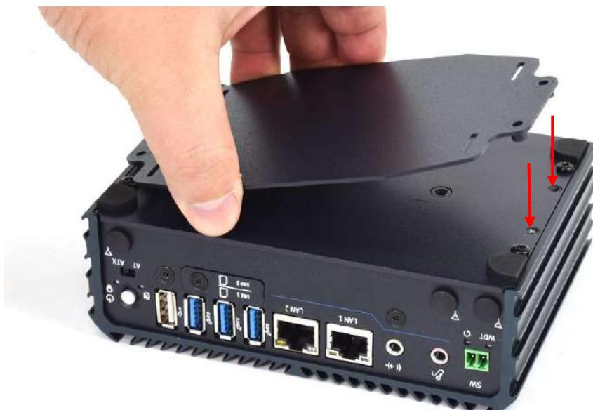
4. Lock the VESA mount kit (for system) with four screws (M3x8L, Nylok).
