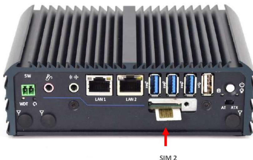
3. Please note that the installation of SIM 1 and SIM 2 has to match the installation of mini PCIe sockets.
