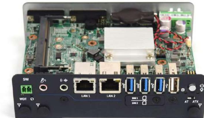
2. Insert memory module from 45 degree direction.
