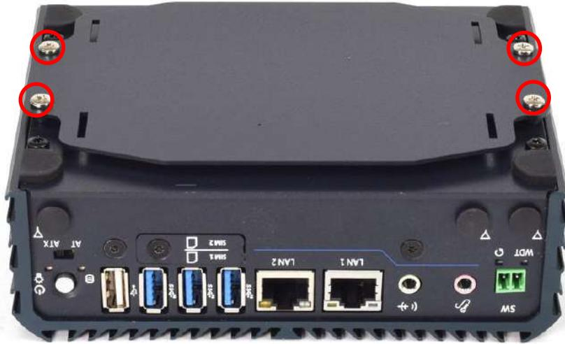
5. VESA mount kit (for panel) should be locked on the back of the panel with four screws.
