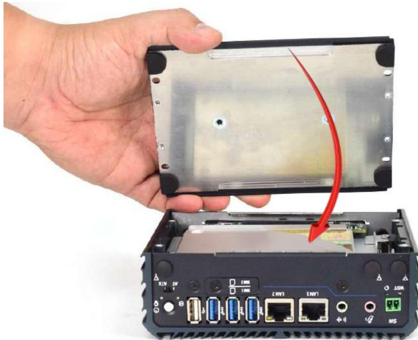
2. Lock the bottom cover with the four screws (M3x5L).
