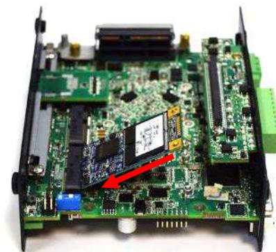
3. Press the mini PCIe card or mSATA module down and lock it with two screws (M2x3.7L).
