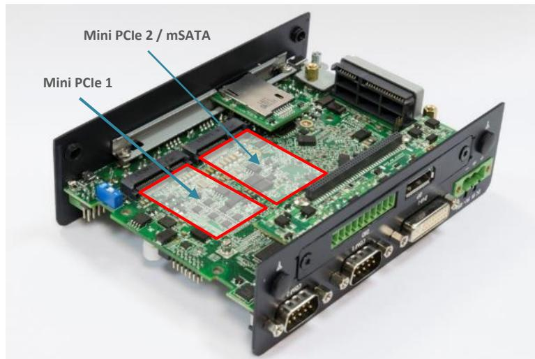
2. Insert mini PCIe card or mSATA module from 45 degree direction.
