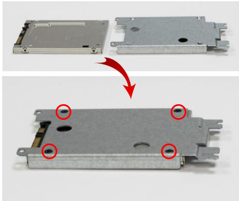
2. Slide the iron plate into the opening on top cover and then place the entire bracket down.
