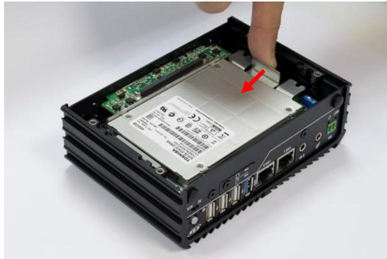
4. Fasten the four screws (M3x5L) to lock the HDD bracket in place.
