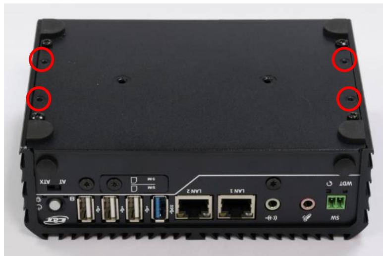
3. Place the side mount kit on top of the system aligning the matching screw holes.
