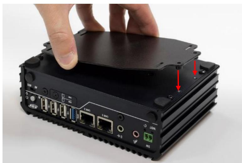
4. Lock the VESA mount kit (for system) with four screws (M3x8L, Nylok).
