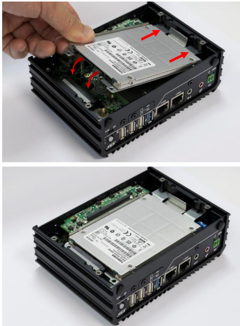
3. Press the entire bracket following the below direction so the SATA connector is firmly plugged into the HDD.
