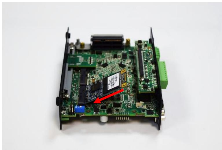
3. Press the mini PCIe card or mSATA module down and lock it with two screws (M2x3.7L).
