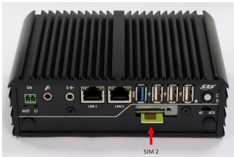
3. Please note that the installation of SIM 1 and SIM 2 has to match the installation of mini PCIe sockets.
