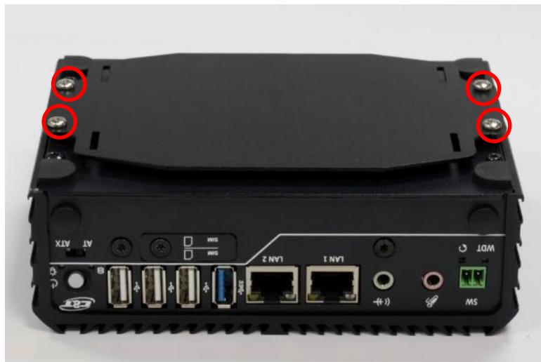
5. VESA mount kit (for panel) should be locked on the back of the panel with four screws.
