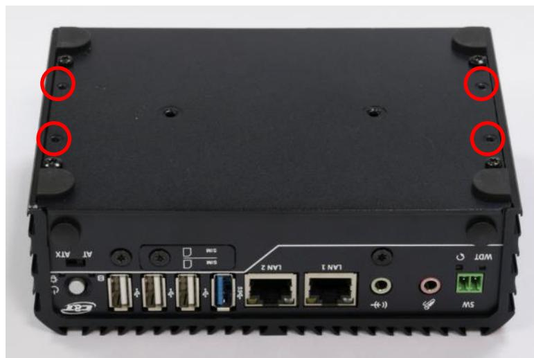
3. Place the VESA mount kit (for system) on top of the system aligning the matching screw holes.
