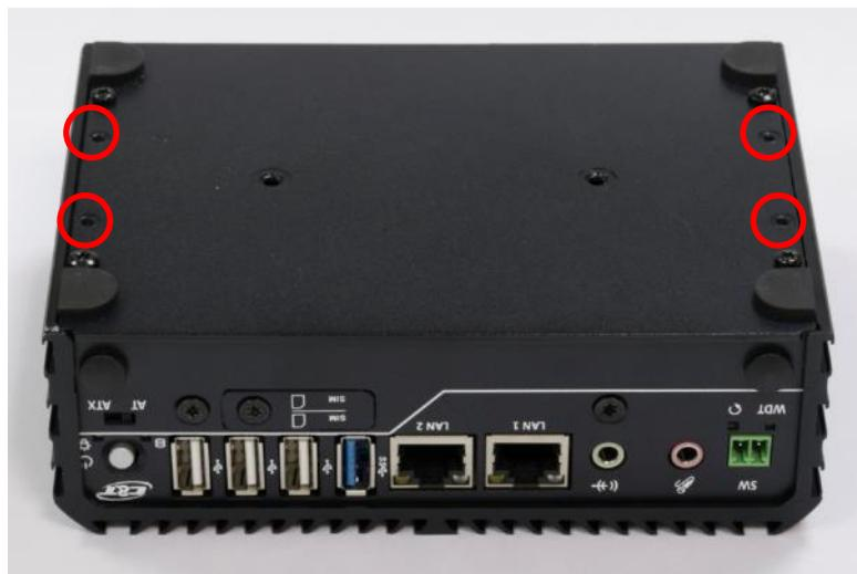
3. Lock the wall mount kit with four screws (M3x5L, Nylok).
