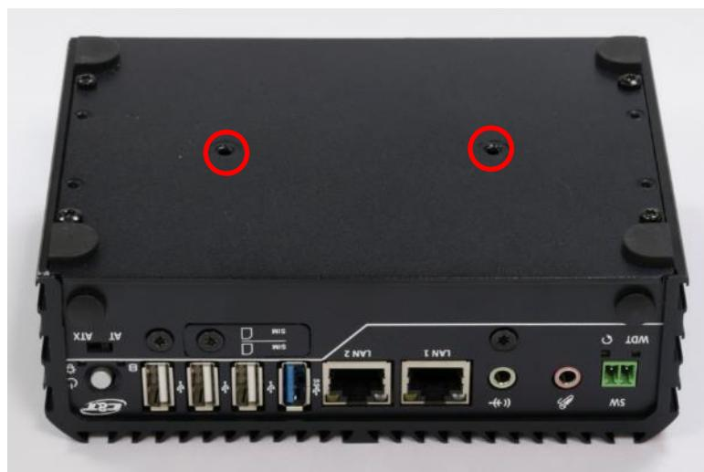
3. Place the din rail holder on top of the bottom cover and lock it with two screws (M4x5L, Nylok).
