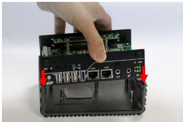
4. Push the system body down until it is firmly in place.
