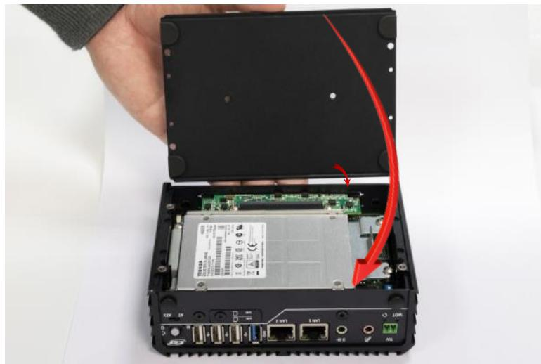
2. Lock the bottom cover with the four screws (M3x5L).
