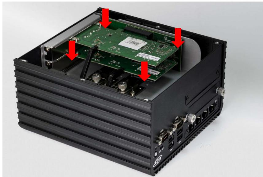
2. Fasten the four screws (M3x5L) below.
