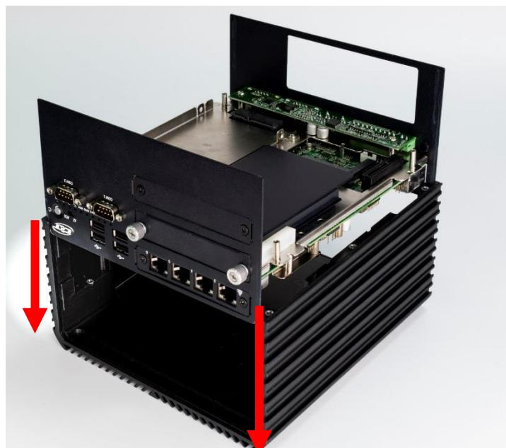
4. Push the system body down until it is firmly in place.
