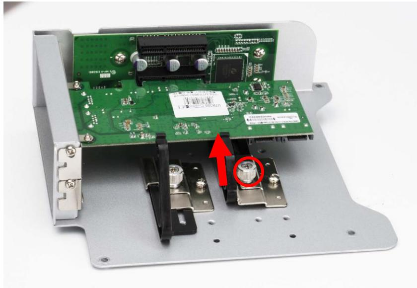
6. For RCO-3022 series, install the upper card (Card 1) first and then install the lower card (Card 2).
