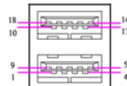
**USB3\_4\_1, USB5\_6\_1, USB7\_8\_1: USB2.0 Connector, Type A**
