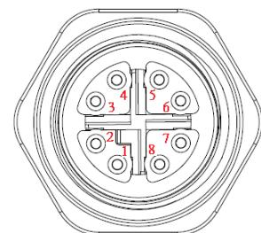
**DC\_IN1: DC Power Input Connector (+9~48V)**
