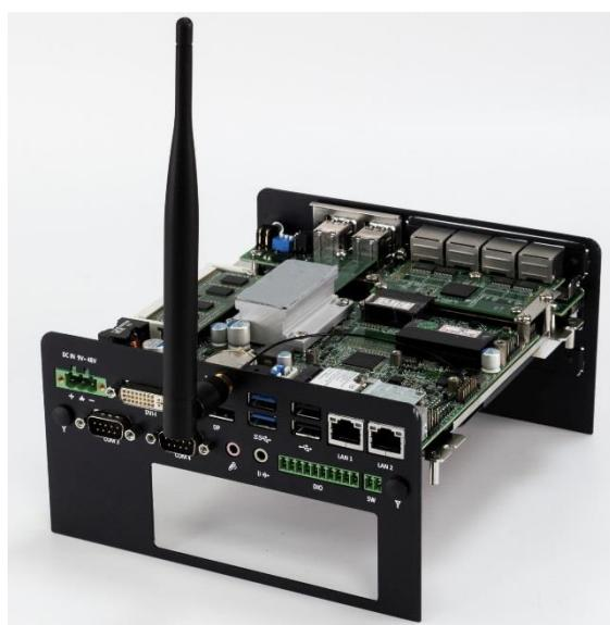
6. Attach the RF connector at the cable-end onto the communication module.
