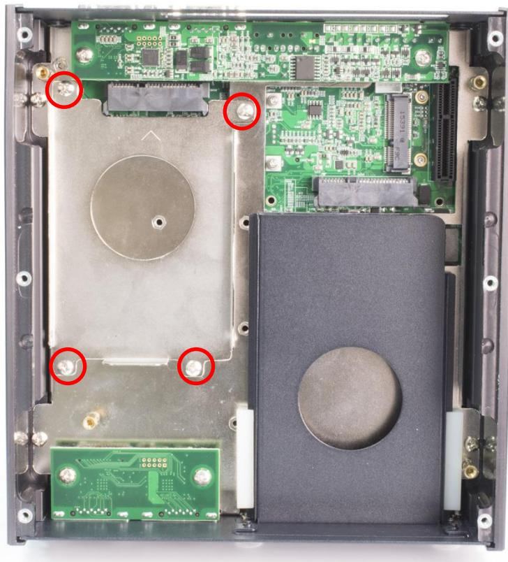
2. Lock the 2.5" HDD with HDD bracket using four screws (M3x4L).
