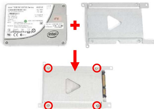
4. Install the HDD bracket following the direction below.
