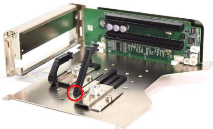
3. Install the PCIe/PCI card according to the below direction and ensure the gold finger is inserted into the slot. Then fasten the screw in the circle.
