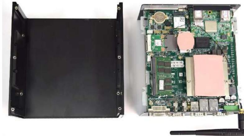
2. Ensure thermal pad is in place on both the CPU thermal block and PCH thermal block.
