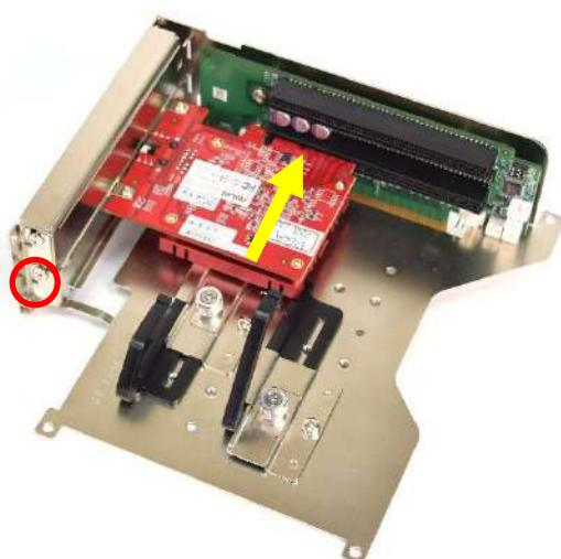
4. Adjust the arm until it holds the card firmly in place. Then fasten the sun screw on the holder. For RCO-3000-CFL-2E series, which has two expansion slots, follow the same procedure to install the second card.
