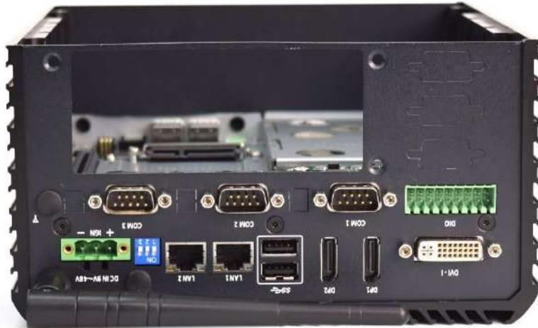
5. Fasten the four screws (M3x5L) to lock the system body with top cover.
