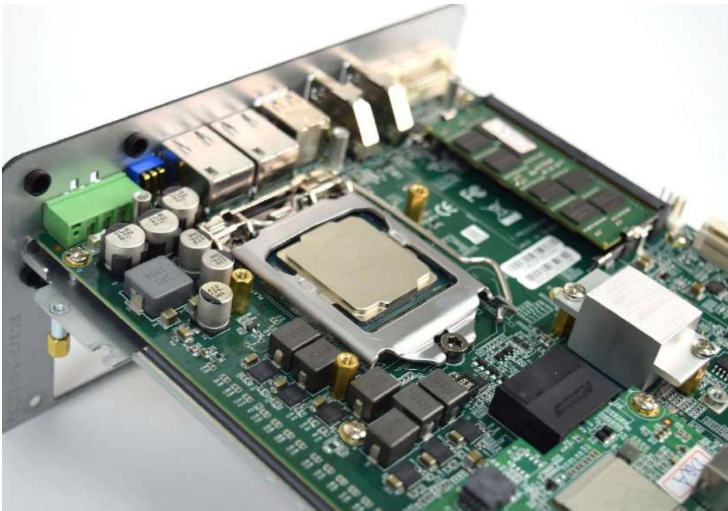
6. Paste thermal pad on the CPU.
