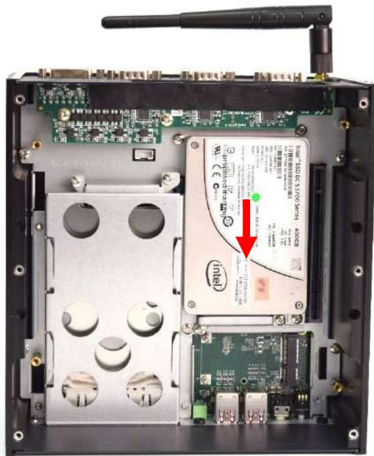
5. Fasten the four screws to lock the internal HDD bracket.
