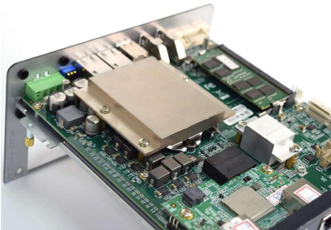
8. Paste the thermal pad onto the installed heat block.
