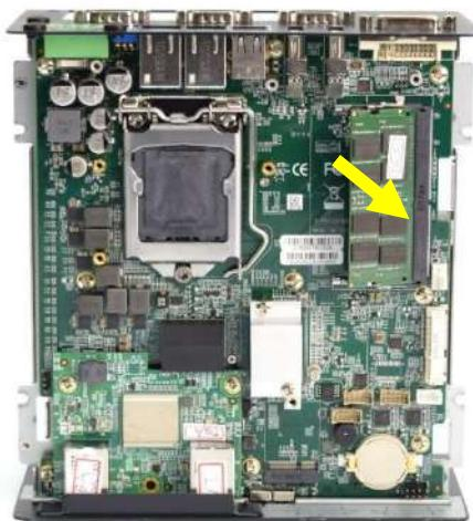
3. Press the memory module vertically downward until you hear the “click” sound. Make sure the memory module is firmly in place.
