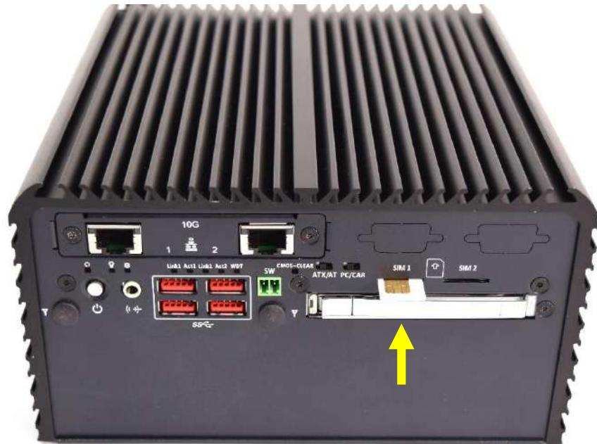
2. Please note that the installation of SIM cards has to match the installation of mini PCIe slots
