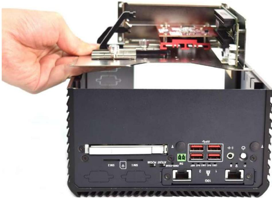
2. Fasten the four screws (M3x5L) below to lock the expansion module.
