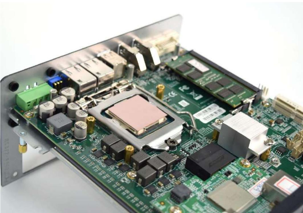
7. Place the designated heat block onto the CPU with thermal pad.
