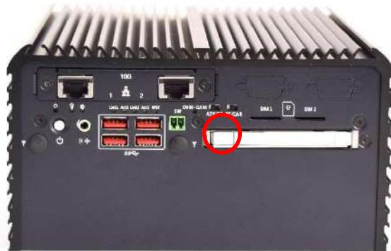
3. Unlock the drive lock and insert the HDD/SSD.
