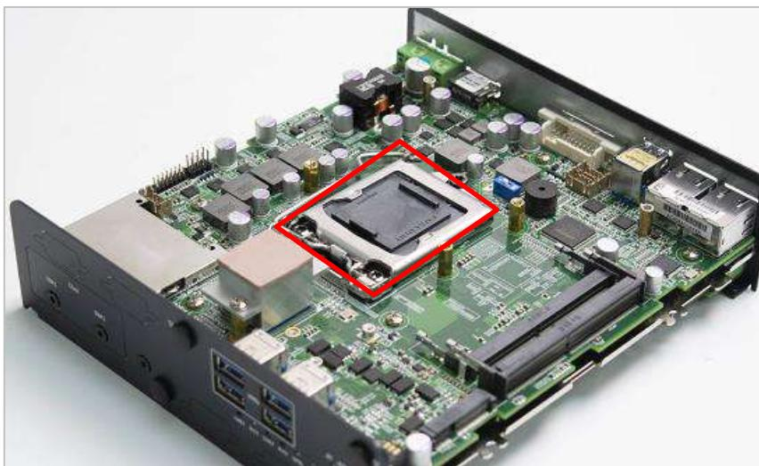
2. Press down the CPU socket lever in order to open the socket cover.
