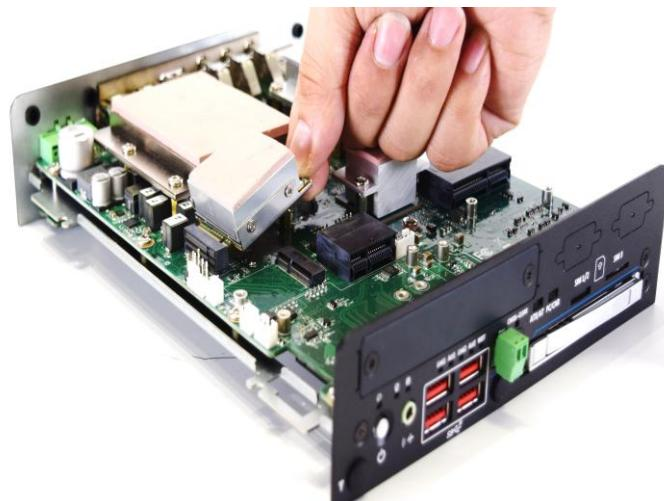
3. Press the 4G/5G card down and secure with one screw (M2x4L).
