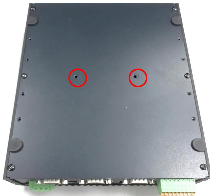
3. Place the din rail holder on top of the bottom cover and secure with two screws (M4x5L, Nylok).
