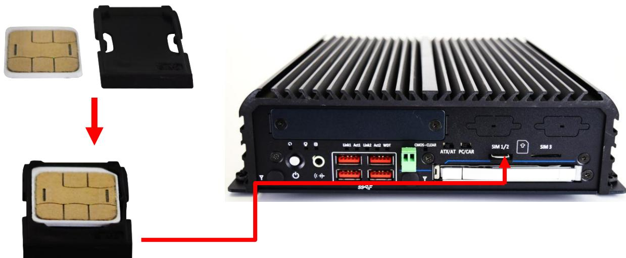
4. Insert SIM card into the socket for SIM3.
