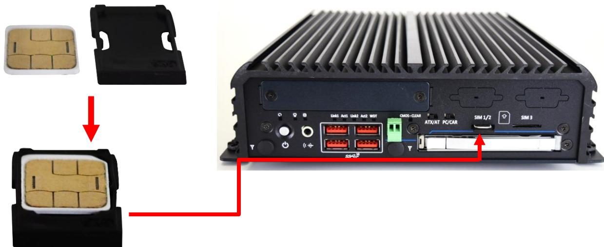
3. Place the Mini SIM card on the back of the tray for SIM2.
