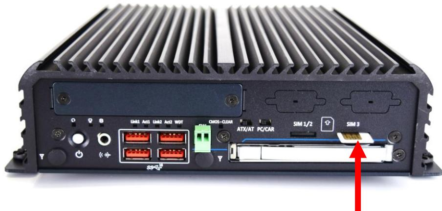
5. Please note that the installation of SIM cards has to match the installation of M.2 B Key slots
