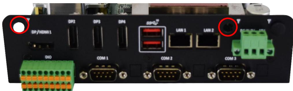
6. Install the SMA female jack through the antenna holes, and then fasten on the SMA male plug.
