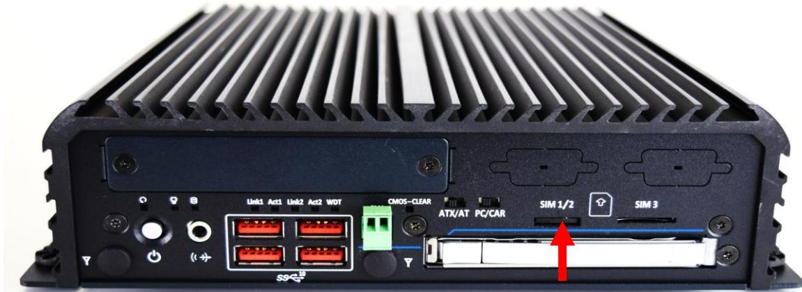
2. Place the Mini SIM card on the front of the tray for SIM1.
