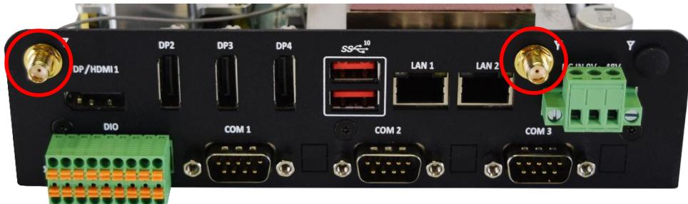
5. Fix the end of the cable of the Wireless RF connector onto the communication module as shown in the picture below.
