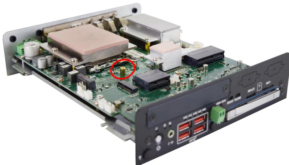
2. Insert 4G/5G card at a 45-degree angle.
