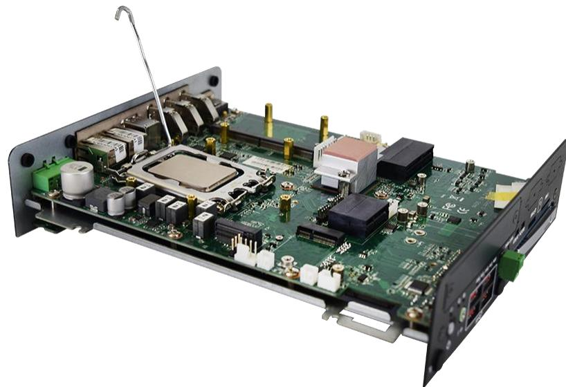
6. Press down the CPU socket lever in order to secure the socket.
