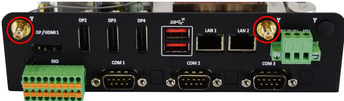
7. Fix the end of the cable of the Wireless RF connector onto the communication module as shown in the picture below.
