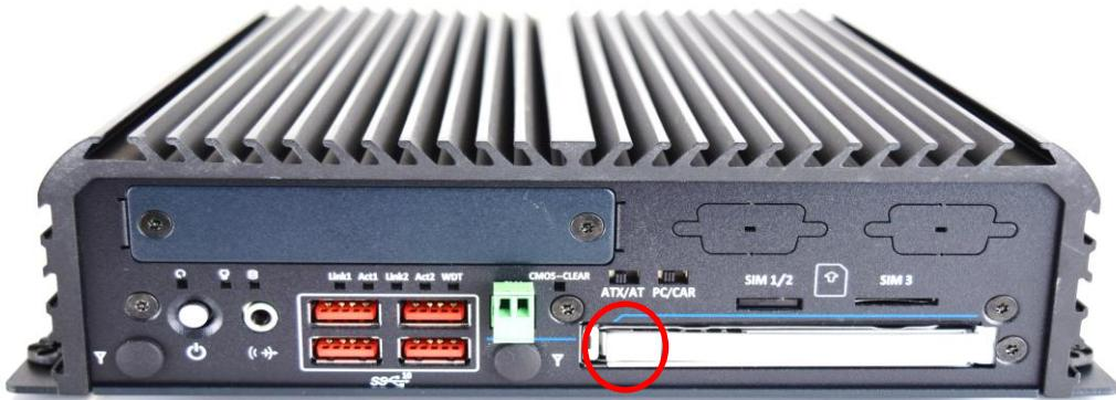
2. Unlock the drive lock and insert the HDD/SSD.
