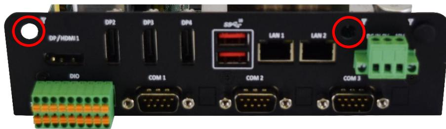
4. Install the SMA female jack through the antenna holes, and then fasten on the SMA male plug.
