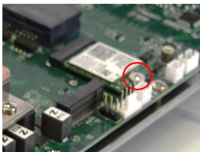
3. Remove antenna hole cover on the system panel.
