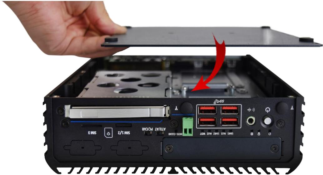
2. Secure the bottom cover with the six screws (M3x5L).
