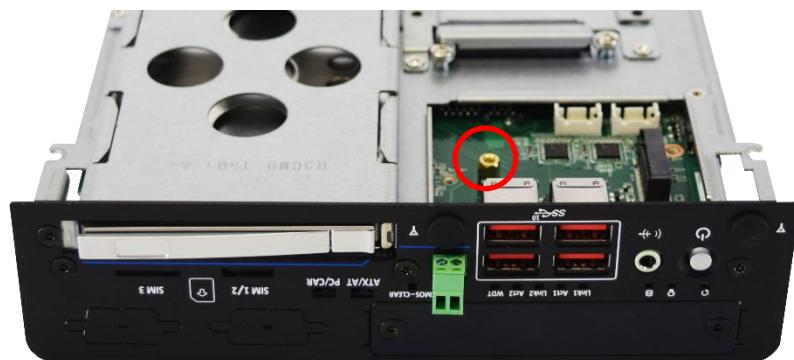
2. Insert 4G/5G card at a 45-degree angle.
