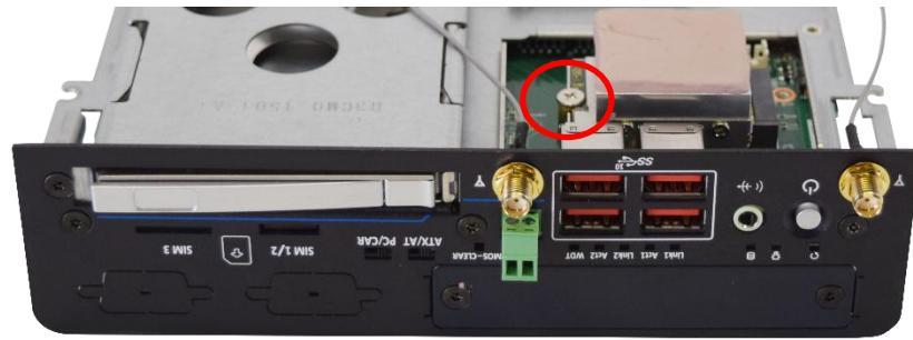
7. Assemble the antenna and SMA jack together, the outcome should look like the picture below.
