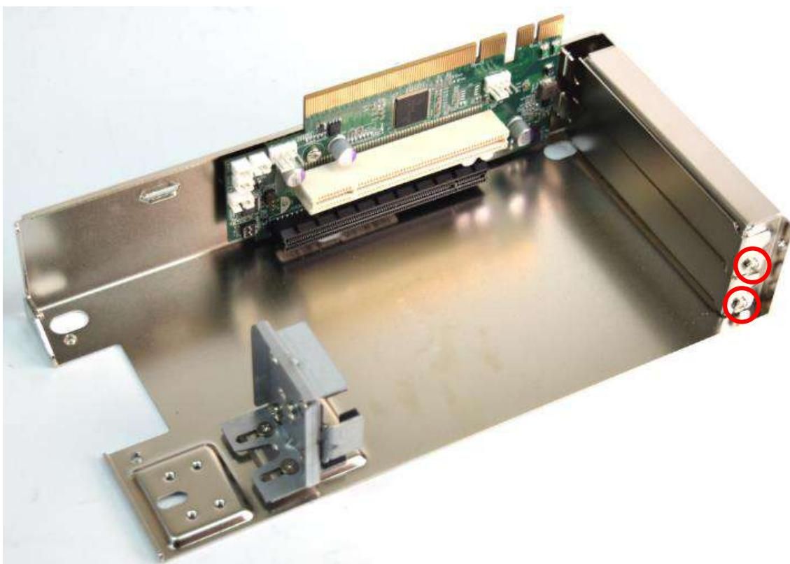
3. Install the PCIe/PCI extension card and ensure the gold finger is inserted into the slot. and then fasten the screw.
