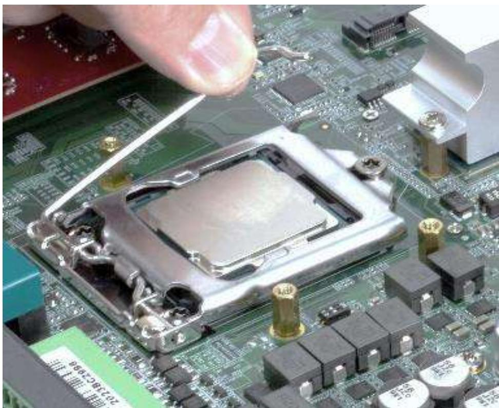
5. Paste thermal pad on the CPU.
