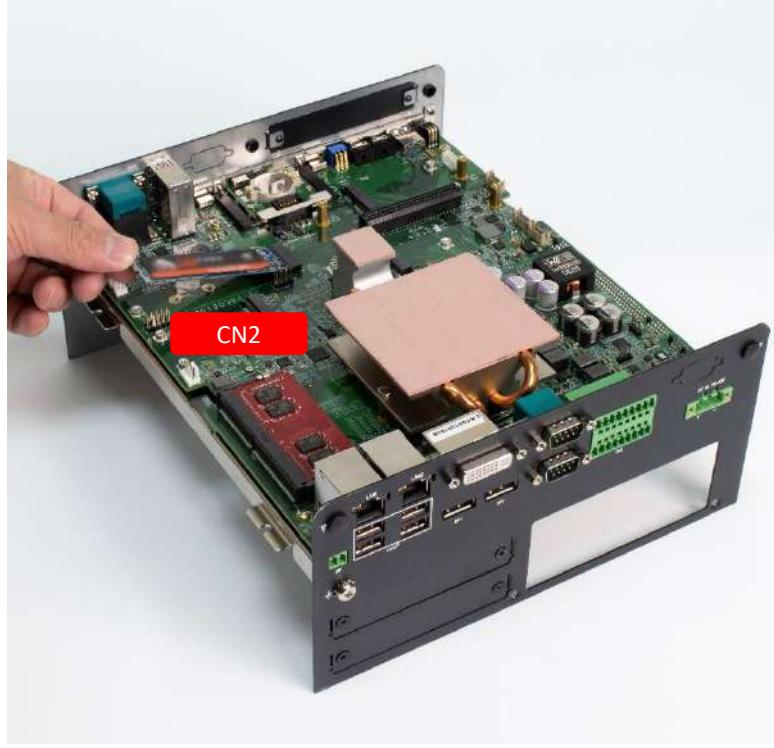
2. Press the M.2 M Key card down and lock it with one screw (M2x3.7L).
