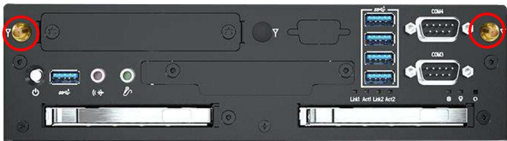
5. Assemble the antenna and SMA jack together.
