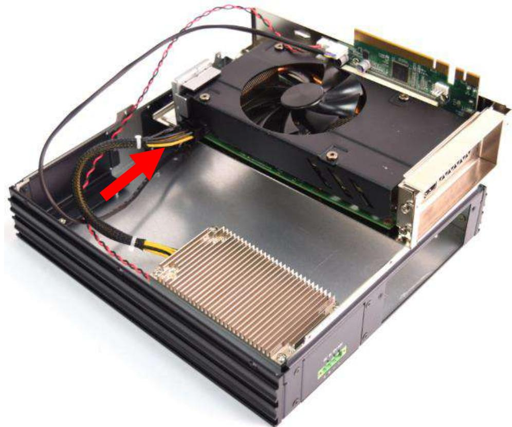
6. Put the graphic expansion module into the expansion chassis.
