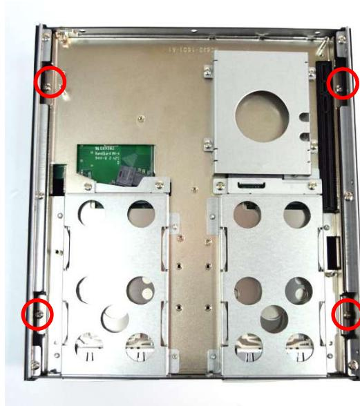
2. Hold the body of the system and lift it vertically away from the top cover.
