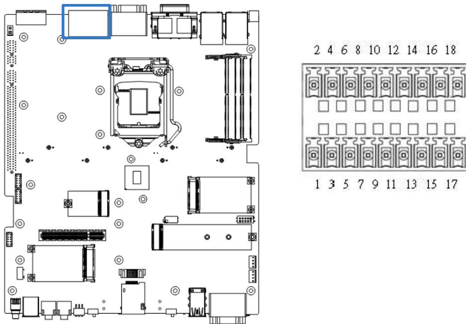
**DIO : Digital Input / Output Connector Type: Terminal Block 2x9 18-pin, 3.5mm pitch**
