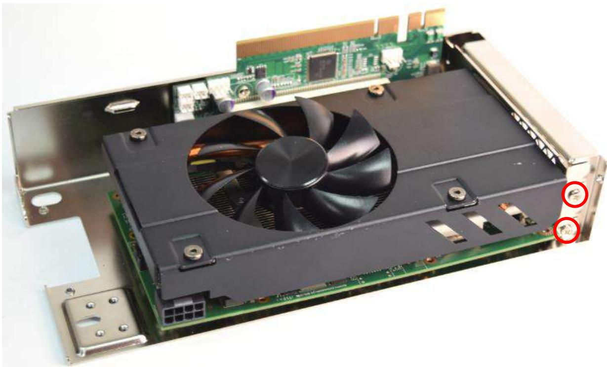
4. Adjust the arm until it holds the card firmly in place. Then fasten the screw on the holder.
