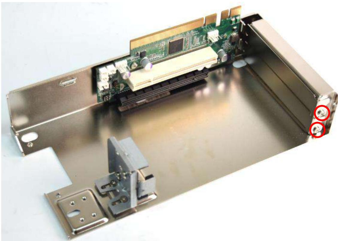
2. Unscrew the card bracket screws to remove the bracket from the expansion slots
