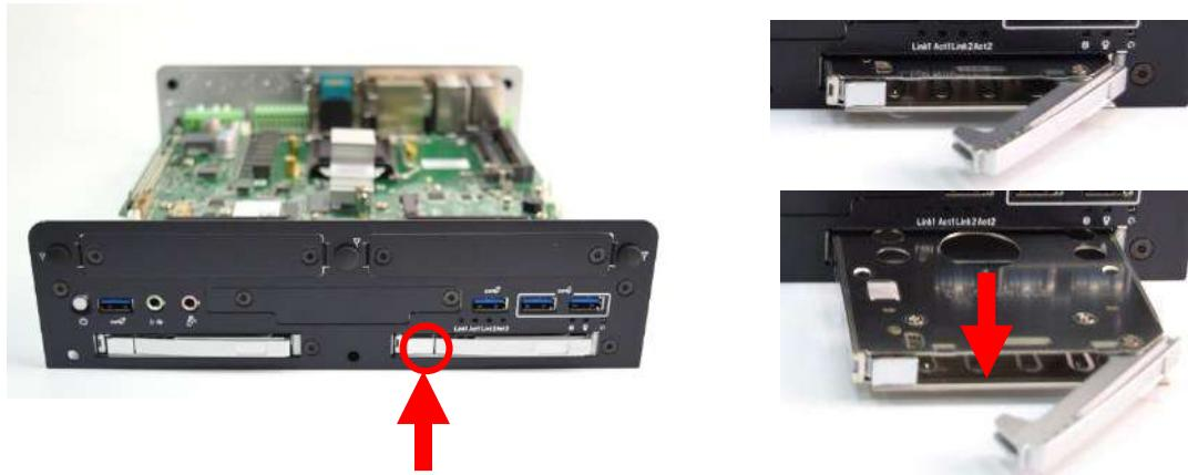
2. Unlock the drive lock (red circle) and insert the HDD/SSD.
