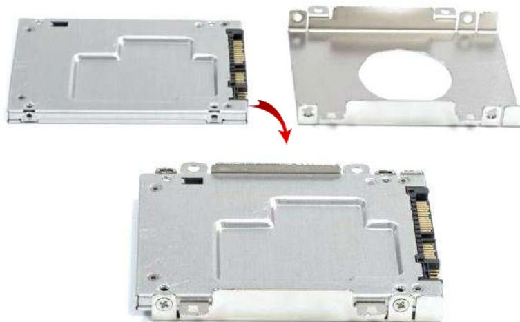
3. Install the HDD/SSD bracket following the direction below.
