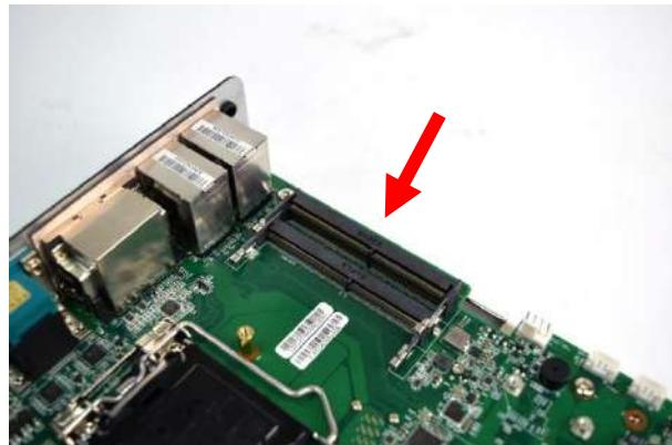
2. Insert memory module from 45 degree direction.
