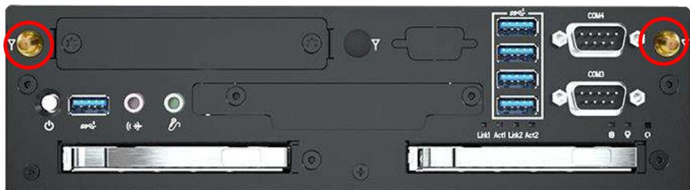
3. Assemble the antenna and SMA jack together.
