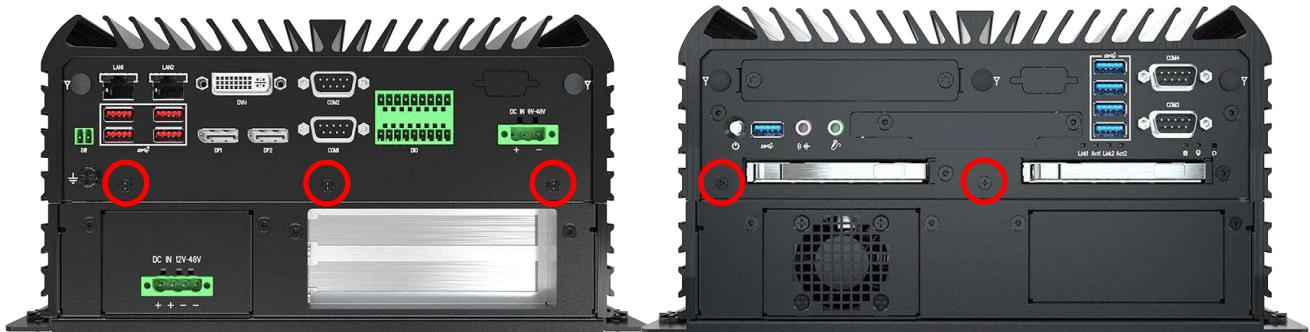
3. Now you can separate the expansion module from the computing module.
