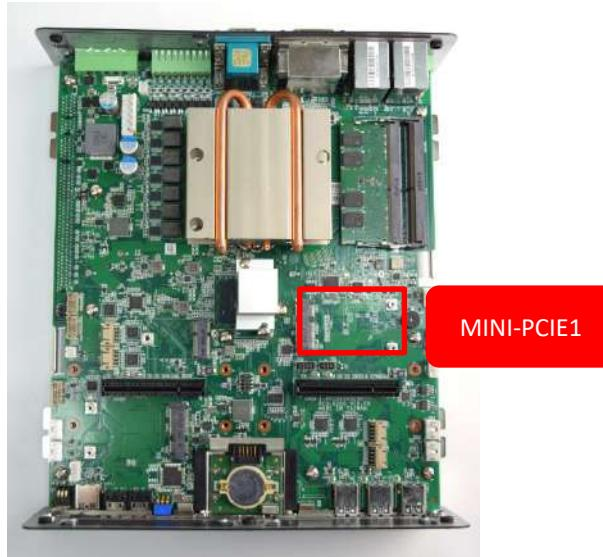
1. Insert Mini PCIe card from 45 degree direction.
