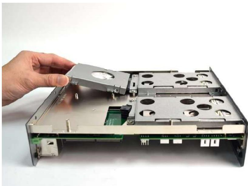
4. Fasten the 4 screws to lock the internal HDD/SSD bracket.
