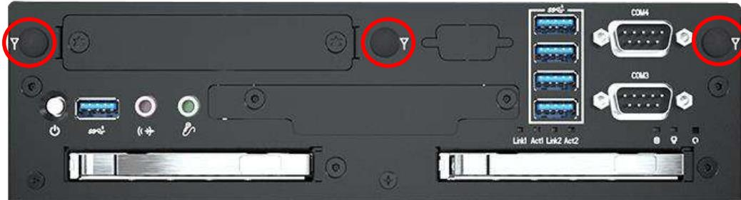
2. Have antenna jack penetrate through the hole, and fasten the nut with SMA jack
