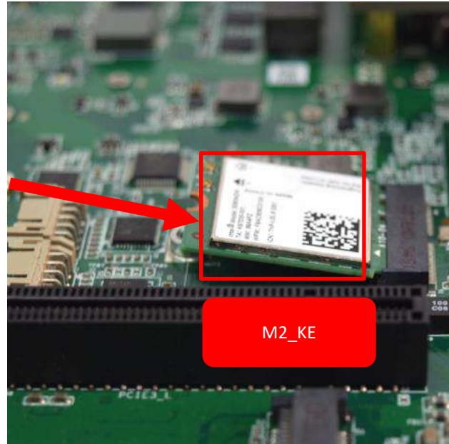
2. Press the M.2 E Key card down and lock it with one screw (M2x3.7L).
