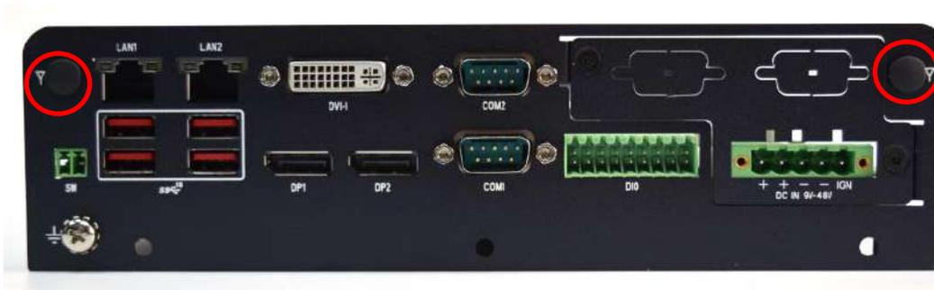
4. Have antenna jack penetrate through the hole, and fasten the nut with SMA jack.
