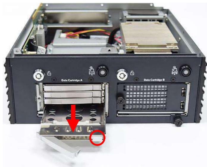
3. Unlock the drive lock and insert the HDD/SSD
