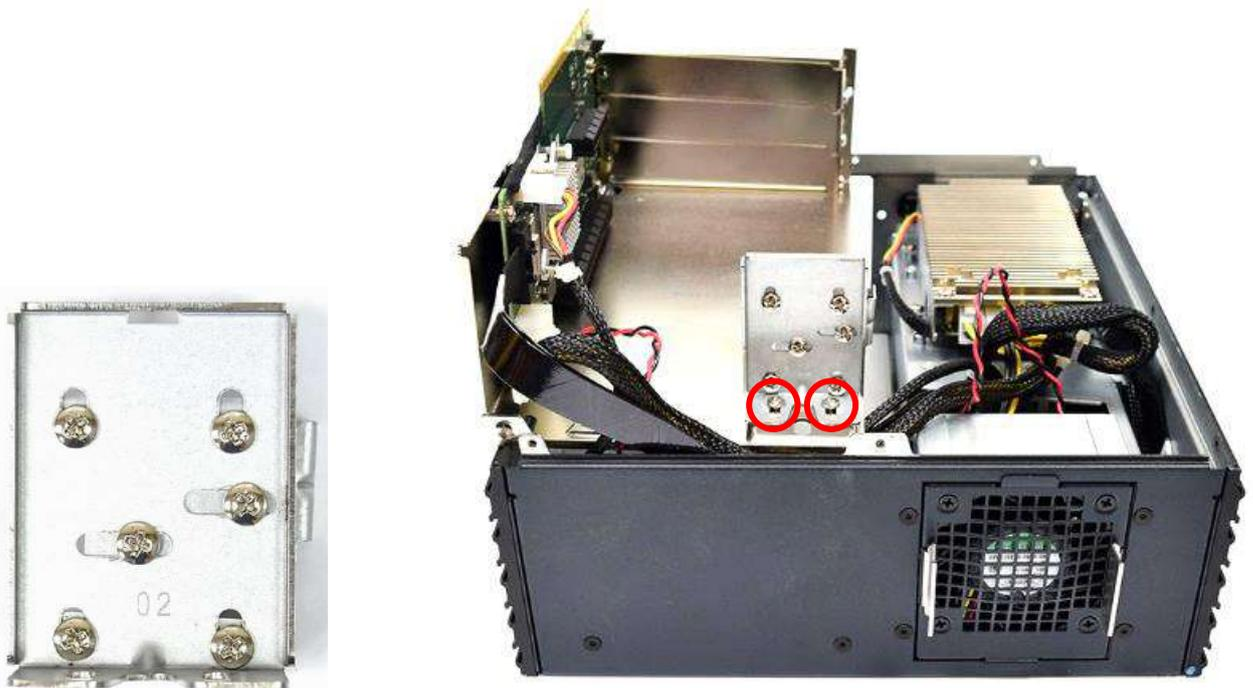
4. Install the graphic card and ensure the gold finger is inserted into the slot. and then fasten the screws.
