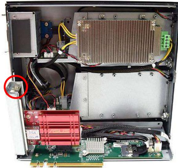
5. Put back the PCIe/PCI expansion card bracket. and then fasten the 5 screws.
