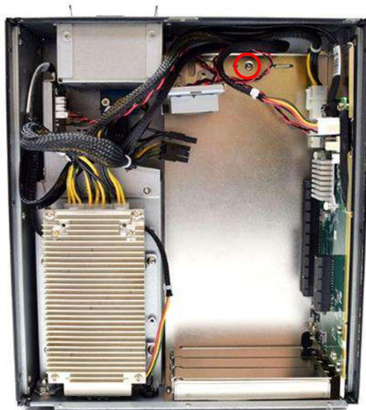
2. Unscrew the 2 screws to remove the I/O shield
