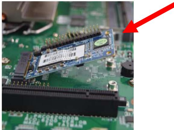
2. Press the Mini PCIe card down and lock it with two screws (M2x3.7L).
