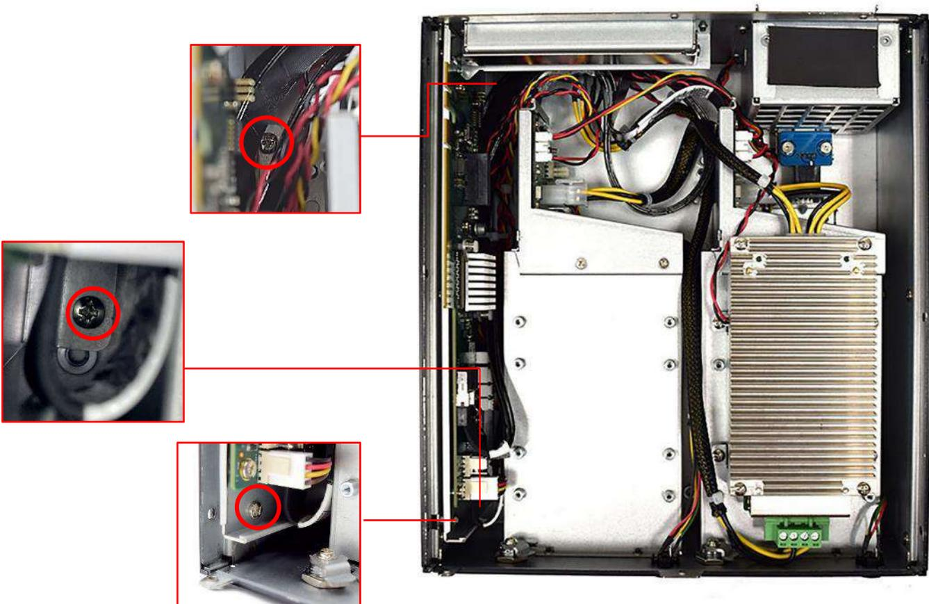
2. Take out the PCIe/PCI expansion card bracket.
