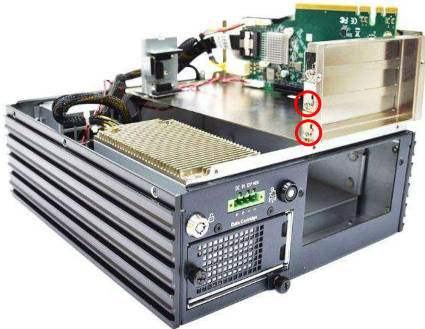
3. Unscrew the card bracket screws to remove the bracket from the expansion slots
