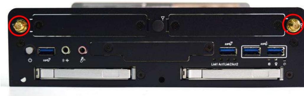
5. Assemble the antenna and SMA jack together.
