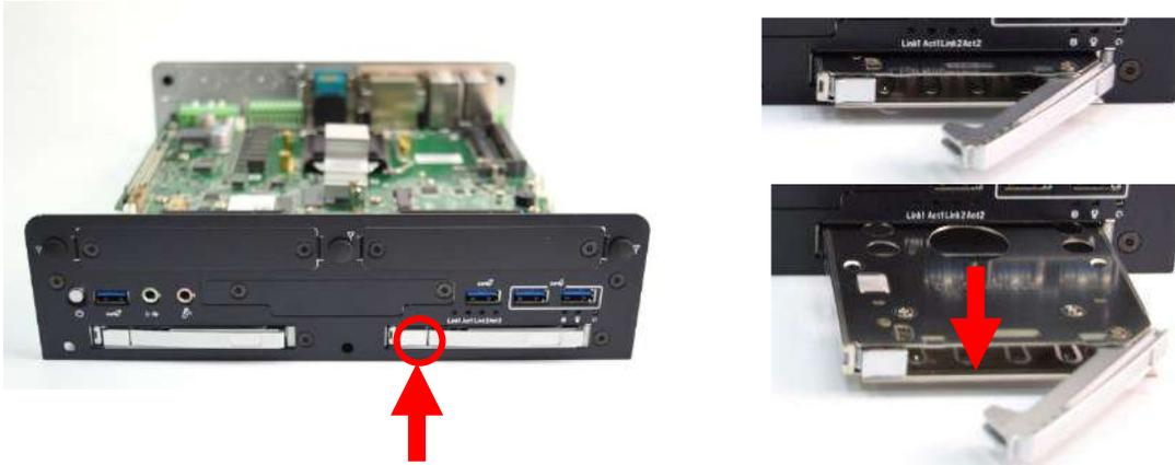
2. Unlock the drive lock (red circle) and insert the HDD/SSD.
