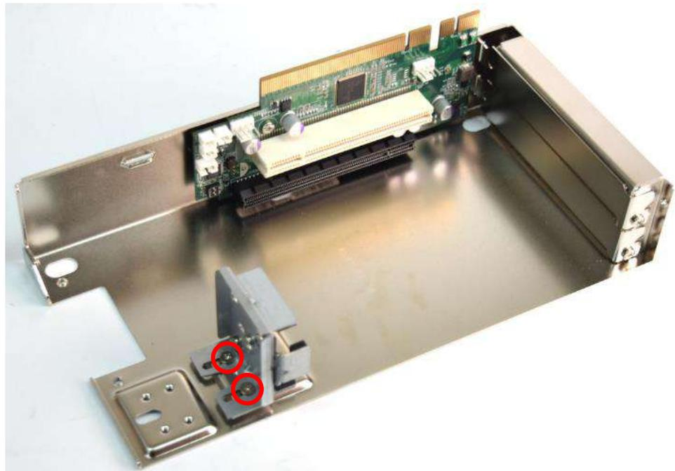
3. Install the graphic card and ensure the gold finger is inserted into the slot. and then fasten the screws.
