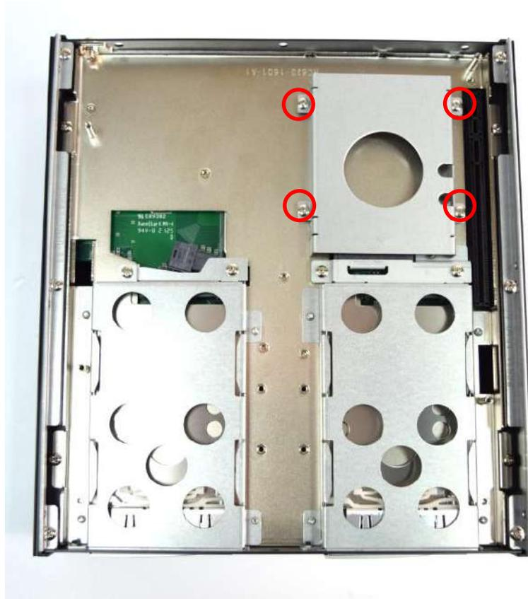
2. Lock the 2.5" HDD with HDD/SSD bracket using four screws (M3x4L).
