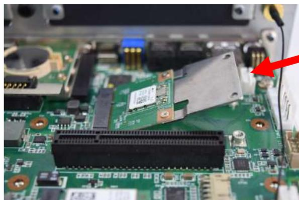
2. Press the Mini PCIe card down and lock it with two screws (M2x3.7L).
