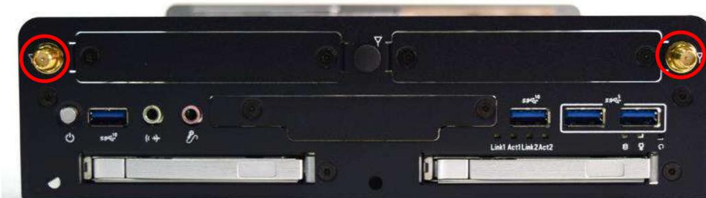
3. Assemble the antenna and SMA jack together.
