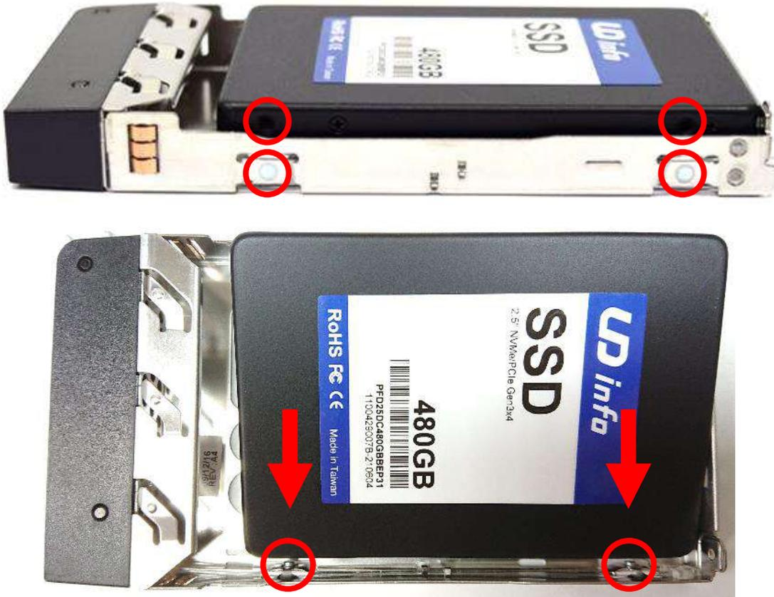
4. Make a little bit force press down another side like the picture shows, has a “click” sound, and the HDD is fully fixed on the HDD tray.
