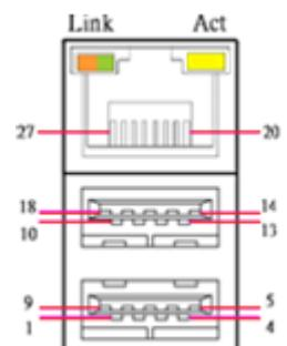
**LAN3, LAN4, LAN5, LAN6, LAN7, LAN8, LAN9, LAN10 : RJ45 with LEDs Port**
