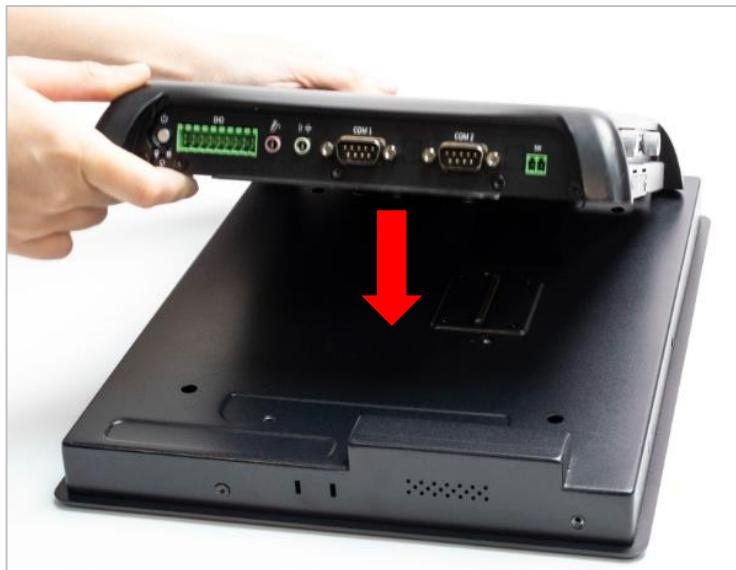
2. Press the PC module downward to ensure two modules are firmly connected.
