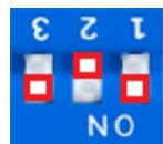
2. The system will shut down 5 minutes later after turning off the vehicle.
