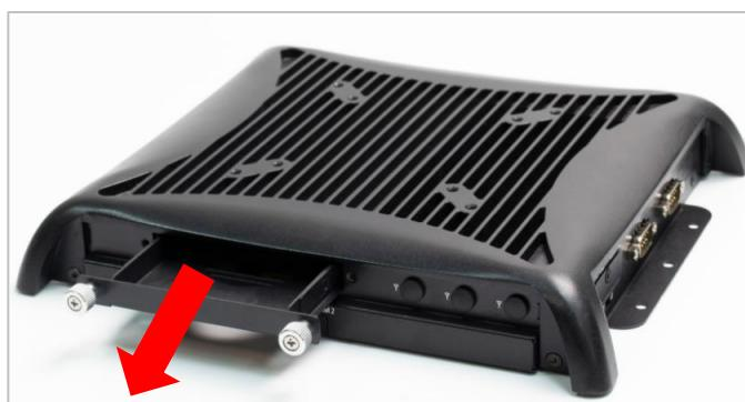
3. Lock the 2.5" HDD with HDD bracket using four screws (M3x4L).
