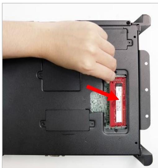
3. Press the memory module vertically downward until you hear the “click” sound. Make sure the memory module is firmly in place.
