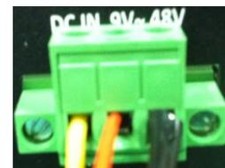
**DC\_IN1: DC Power Input Connector (+9~48V)**
