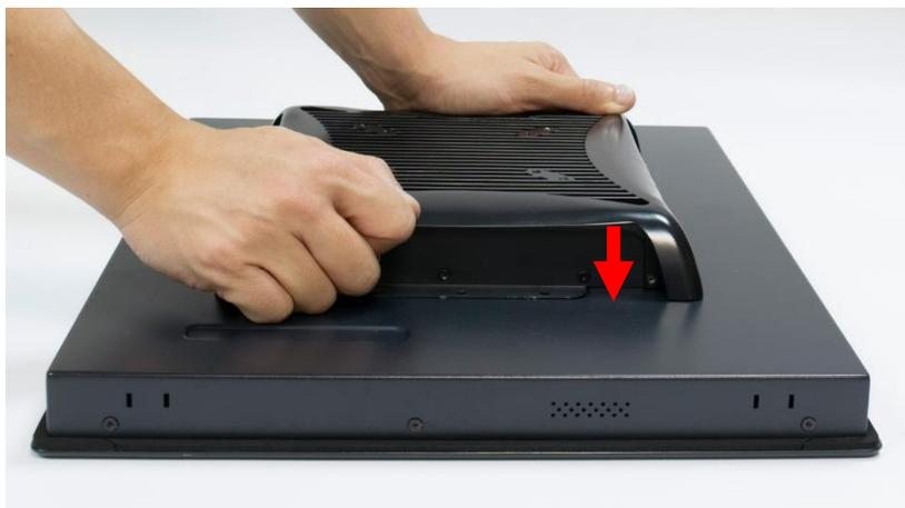
3. Lock the below 6 screws (M4x5L).
