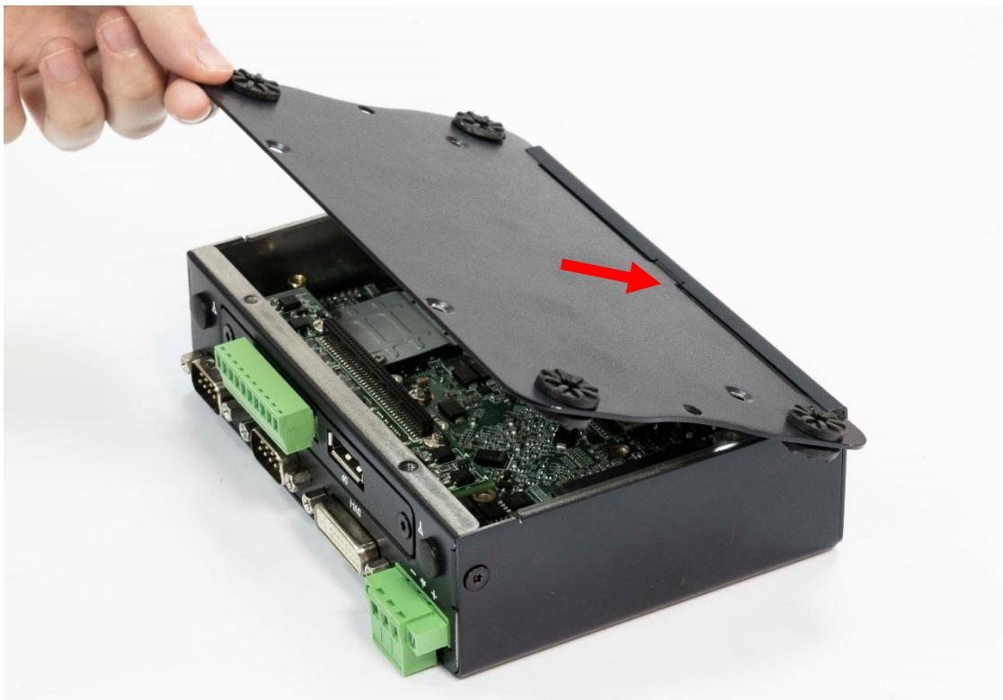
2. Lock the bottom cover with the four screws.
