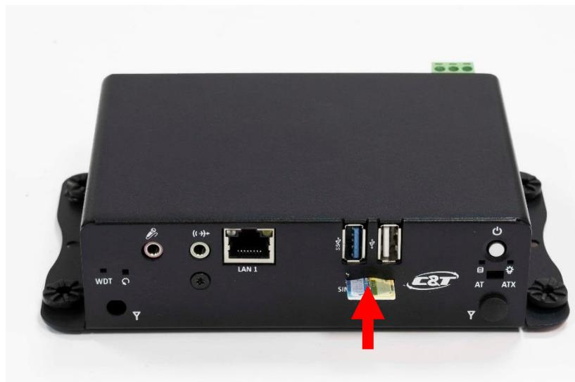
3. To uninstall SIM card, simply press the installed SIM card and then the card will be pushed out.
