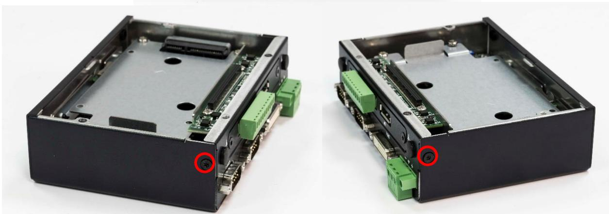
2. Hold the chassis top cover. Pull the system main body following the below direction so the top cover can be separated from it.
