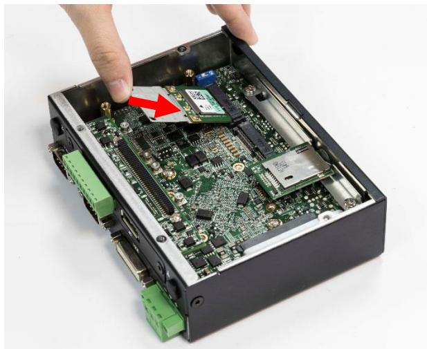
3. Press the mini PCIe card or mSATA module down and lock it with two screws.
