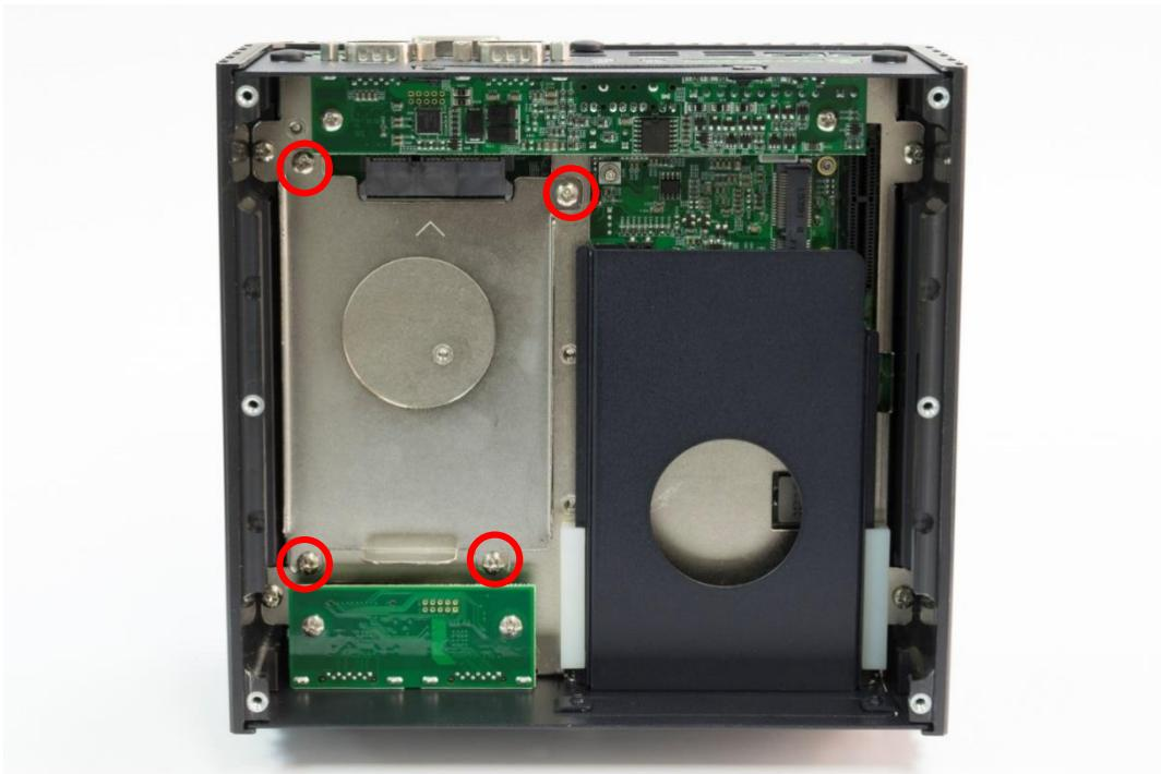
2. Lock the 2.5" HDD with HDD bracket using four screws (M3x4L).
