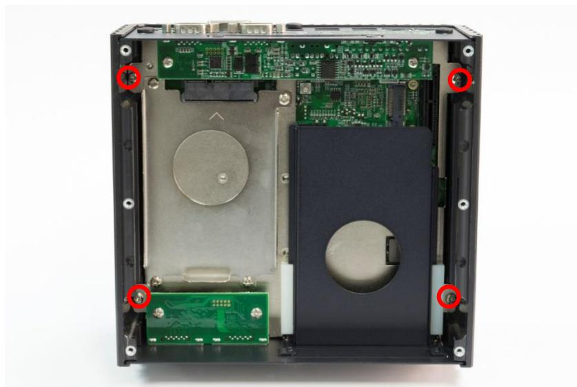
2. Hold the body of the system and lift it vertically away from the top cover.
