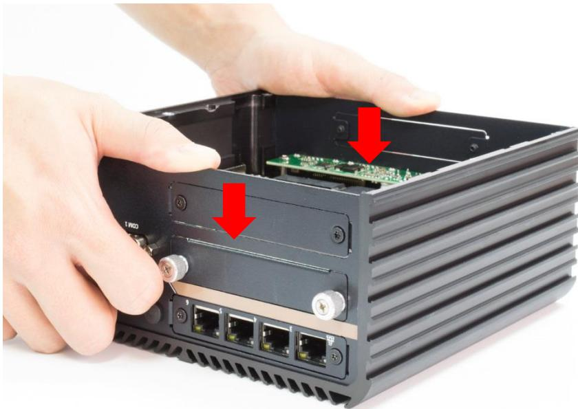
5. Fasten the four screws (M3x5L) to lock the system body with top cover.
