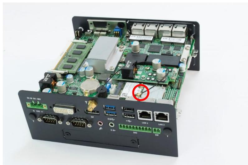
6. Assemble the antenna and antenna jack together.
