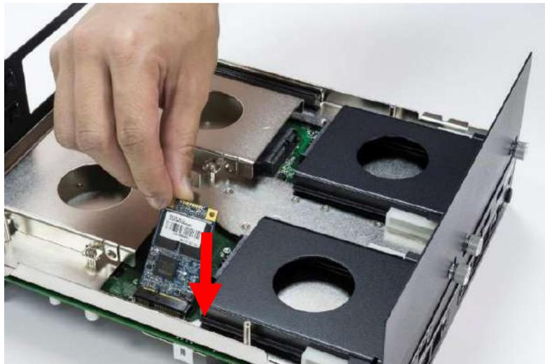
3. Press the mini PCIe card down and lock it with two screws (M2x3.7L).
