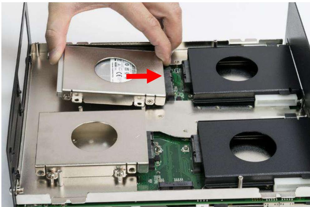
5. Fasten the four screws to lock the internal HDD bracket.
