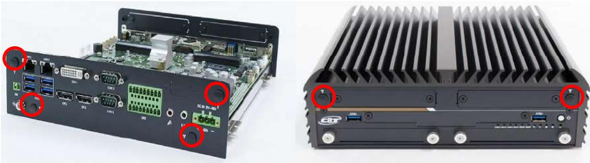
2. Remove antenna hole cover on the system panel.
