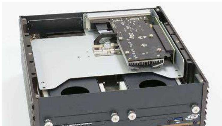
2. Fasten the four screws (M3x5L) below to lock the expansion module.
