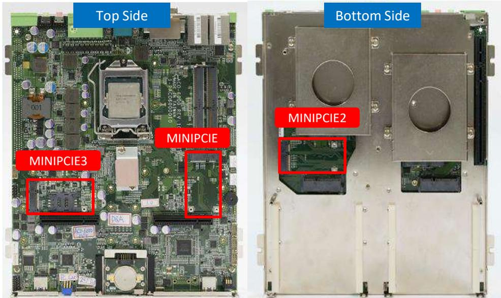
2. Insert mini PCIe card from 45 degree direction.
