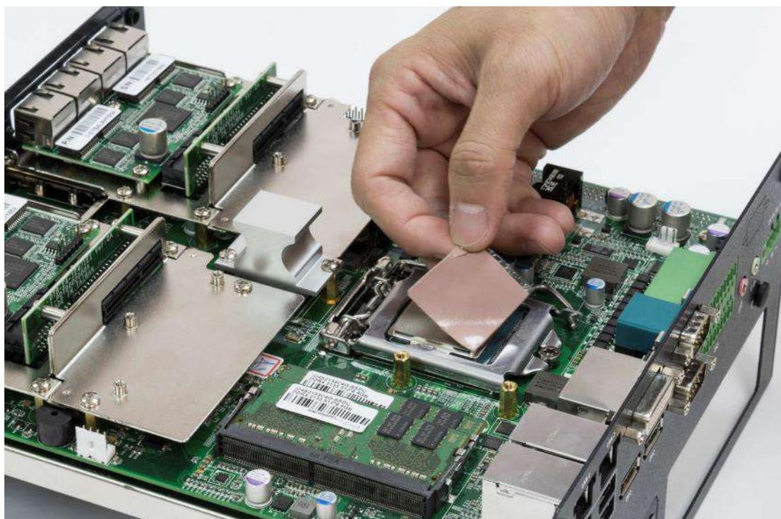
7. Place the designated heat block onto the CPU with thermal pad.
