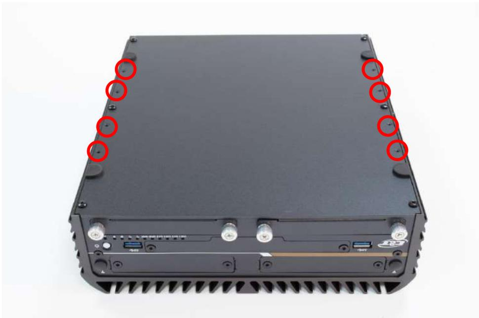
3. Lock the wall mount kit with eight screws (M3x5L, Nylok).
