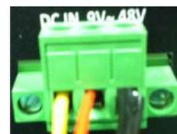
**\* System power On/Off signal must be generated by car ignition, don't manually shut down after ignition off.**
