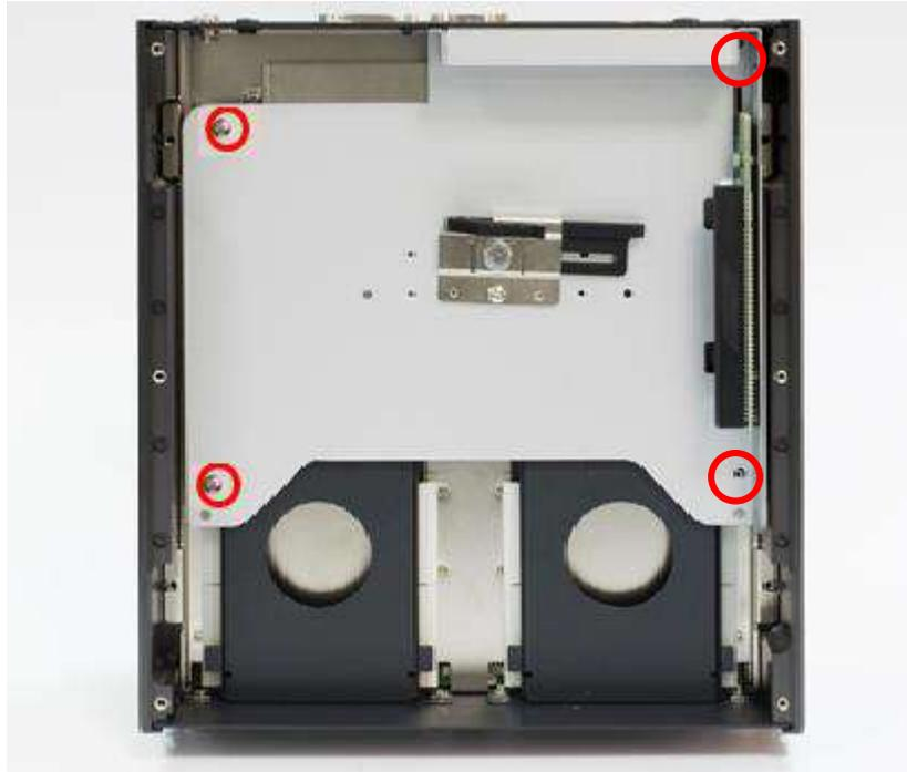
3. Now you can remove the PCIe/PCI expansion module.
