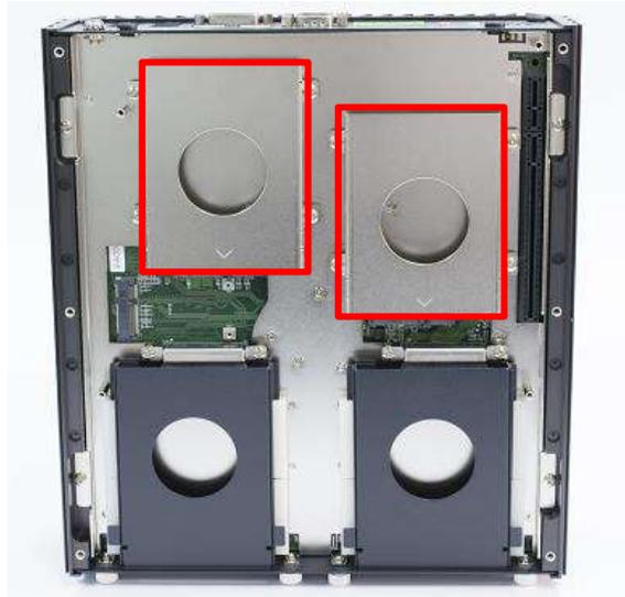
2. Unscrew the four screws (M3x5L) to remove the internal SATA HDD bay.
