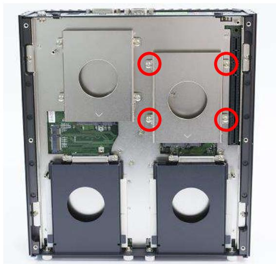
3. Lock the 2.5" HDD with HDD bracket using four screws (M3x4L).
