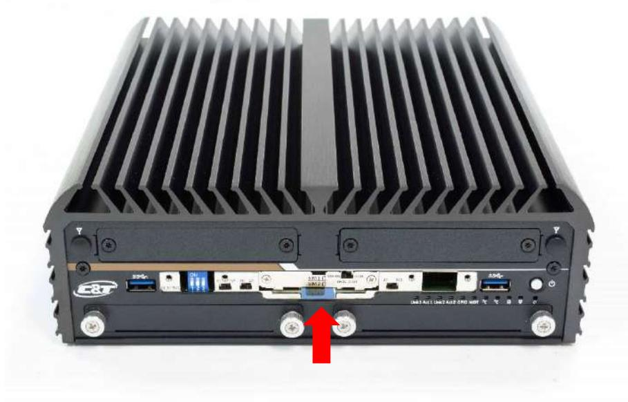
3. Please note that the installation of SIM cards has to match the installation of mini PCIe slots.
