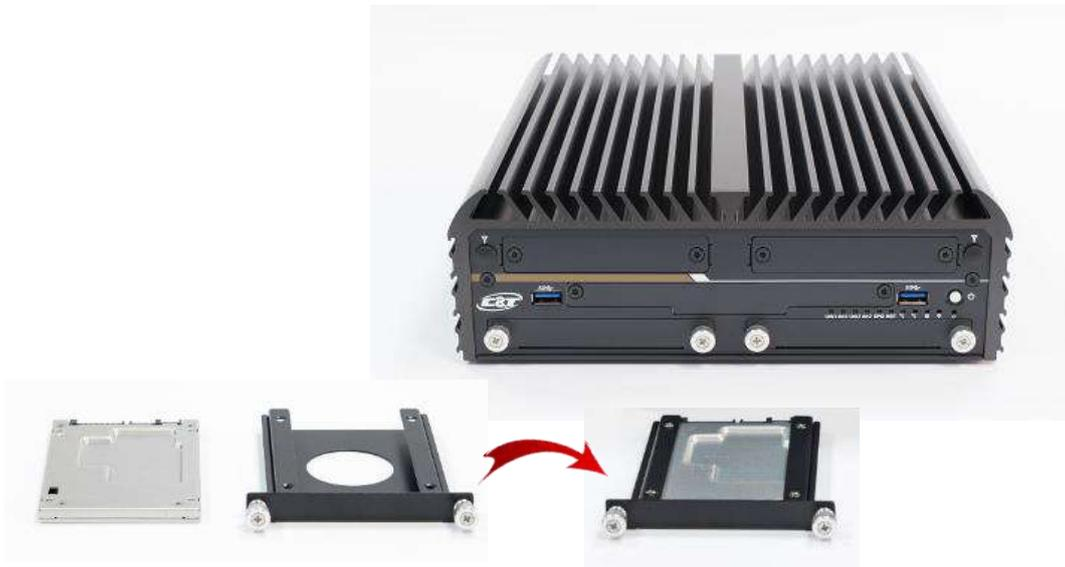
4. Slide the HDD bracket back and then fasten the sun screws.
