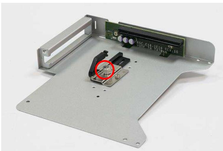
4. Install the PCIe/PCI card according to the below direction and ensure the gold finger is inserted into the slot. Then fasten the screw in the circle.
