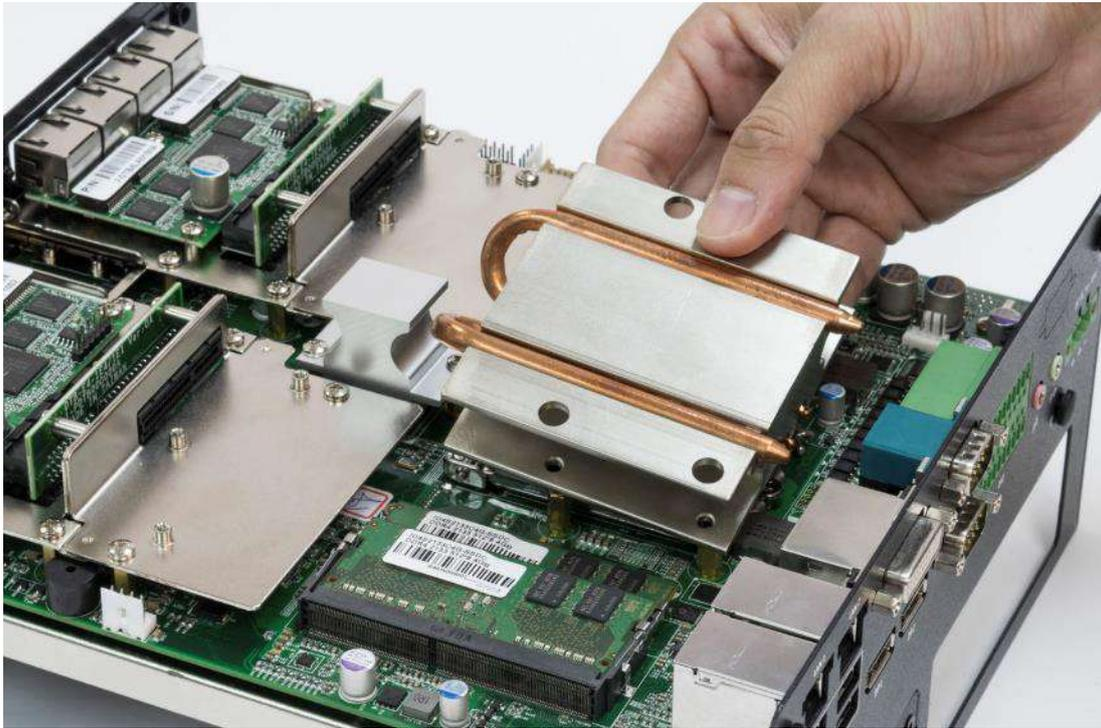
8. Lock the heat block with three screws (M3x5L). Screw driver will be able to penetrate through the holes on the top in order to fasten the screws with copper stud.
