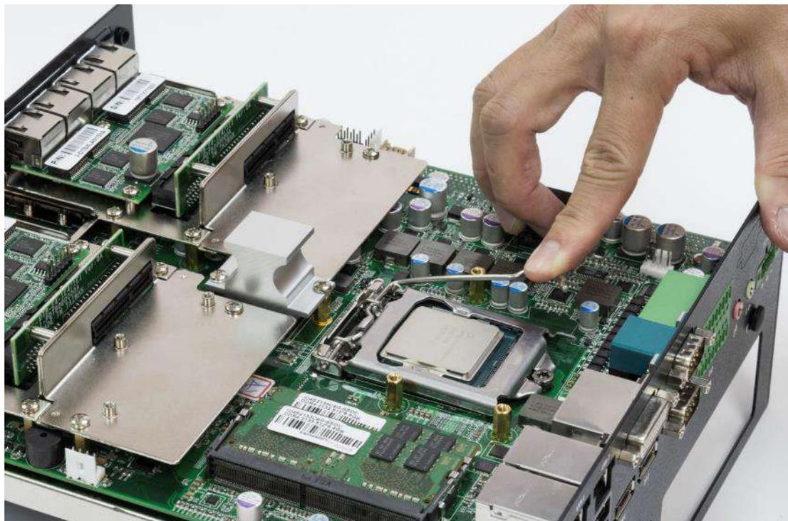
6. Paste thermal pad (1-BR0500040, 29x29x0.5mm) on the CPU.
