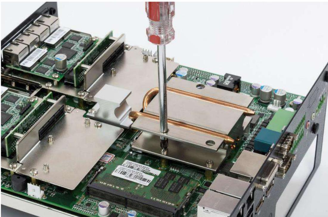
9. Paste the thermal pad (1-BR0500041, 76x70x2.0mm) onto the installed heat block.
