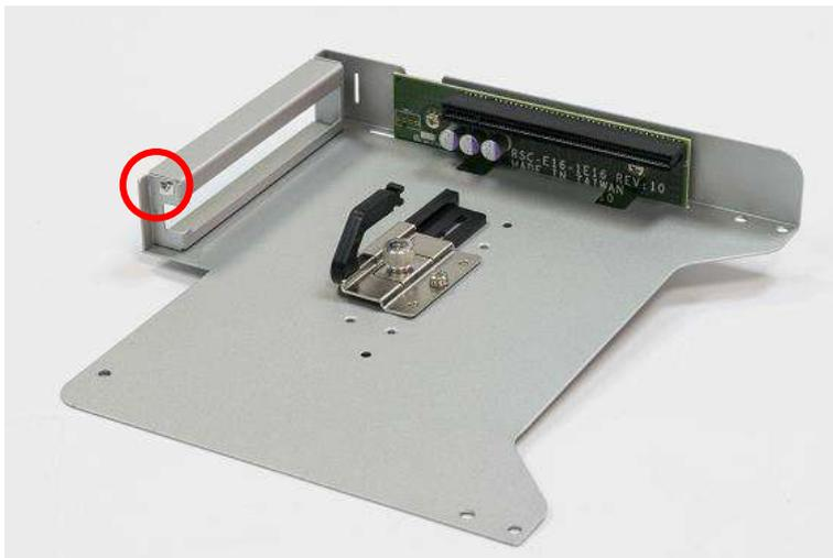
3. Loose the sun screw (circled below) on the holder so the pairing arm can be adjustable.
