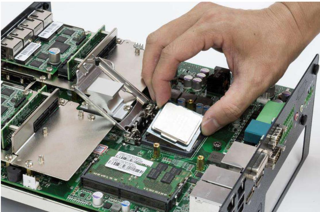
5. Press down the lever again to hold the socket cover.
