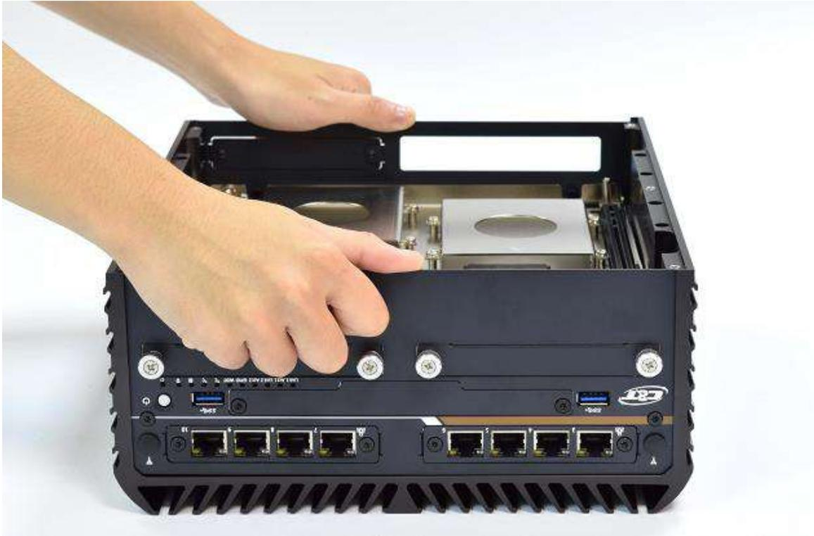
5. Fasten the four screws (M3x5L) to lock the system body with top cover.
