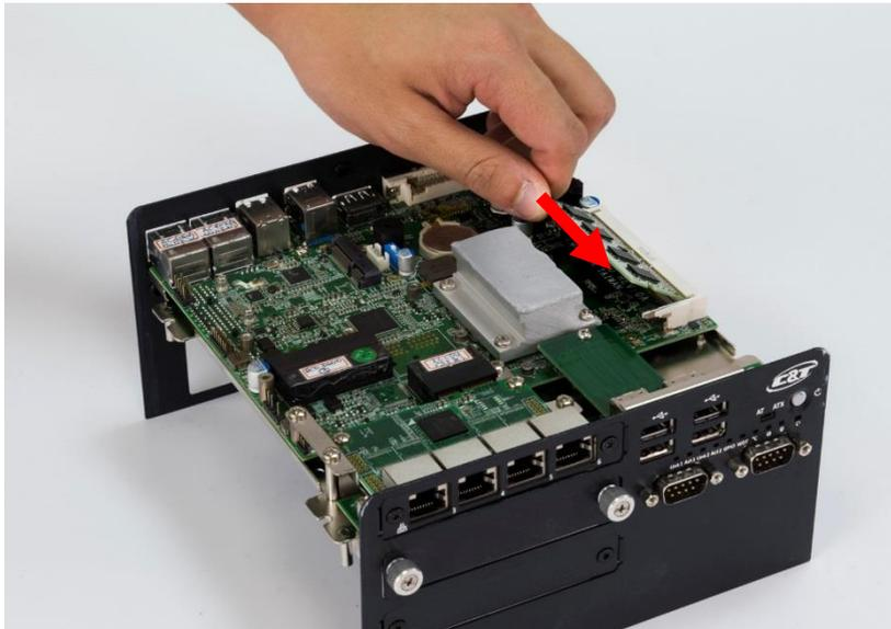
3. Press the memory module vertically downward until you hear the "click" sound. Make sure the memory module is firmly in place.
