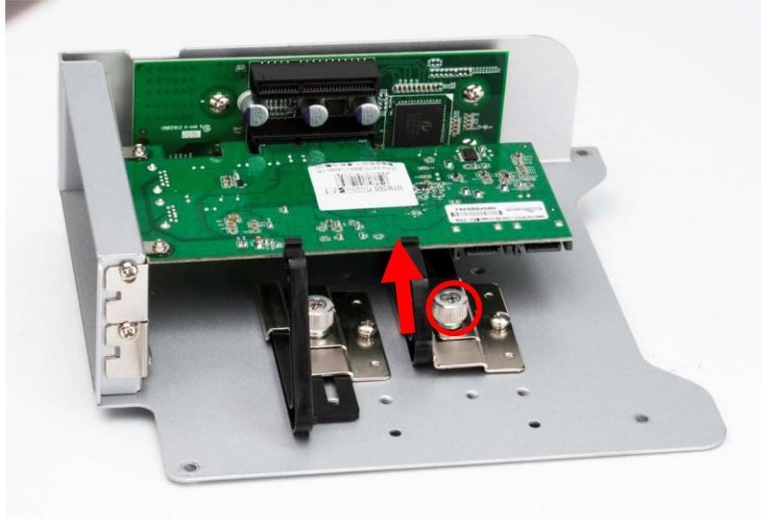
6. For RCO-3022 series, install the upper card (Card 1) first and then install the lower card (Card 2).
