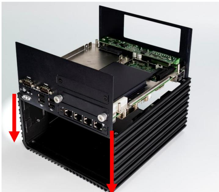
4. Push the system body down until it is firmly in place.
