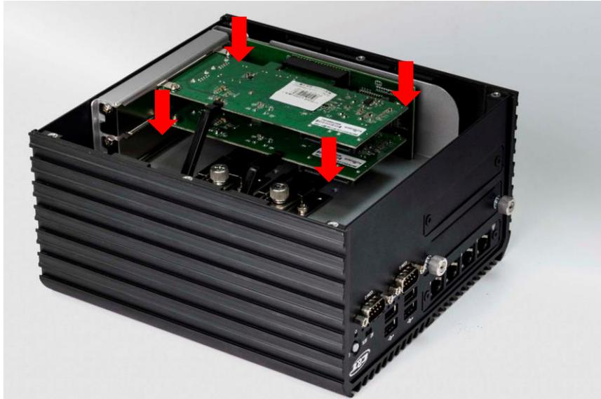
2. Fasten the four screws (M3x5L) below.
