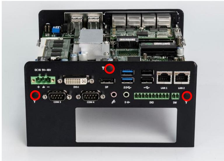
2. Remove antenna hole cover on the system panel.
