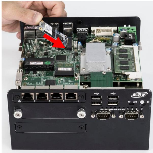
3. Press the mini PCIe card or mSATA module down and lock it with two screws (M2x3.7L).
