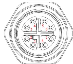
**DC\_IN1: DC Power Input Connector (+9~48V)**
