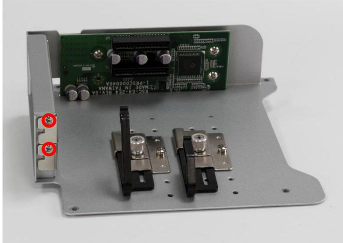
3. Loose the sun screw (circled below) on the holder so the pairing arm can be adjustable.
