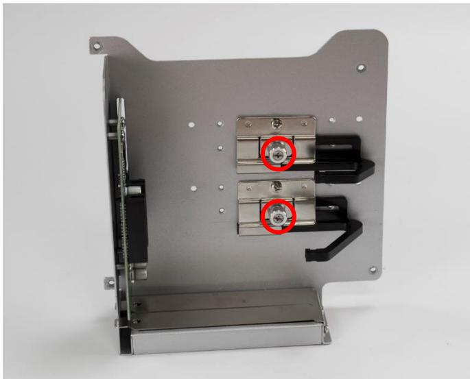
4. Install the PCIe/PCI card according to the below direction and ensure the gold finger is inserted into the slot. Then fasten the screw in the circle.
