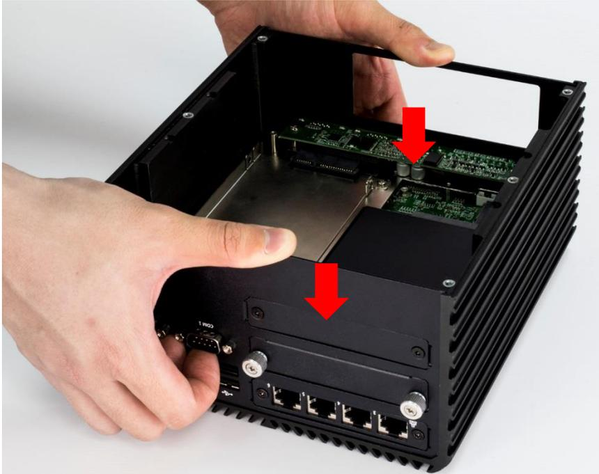
5. Fasten the six screws (M3x5L) to lock the system body with top cover.
