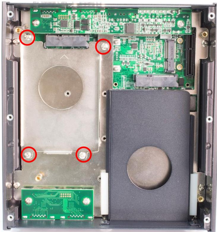
2. Lock the 2.5" HDD with HDD bracket using four screws (M3x4L).
