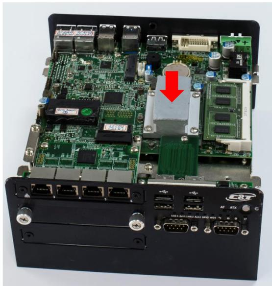
3. Hold the system body and slide the front/rear panel into the slide rail on the top cover.
