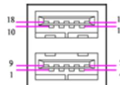
**USB3\_4\_1, USB5\_6\_1, USB7\_8\_1: USB2.0 Connector, Type A**
