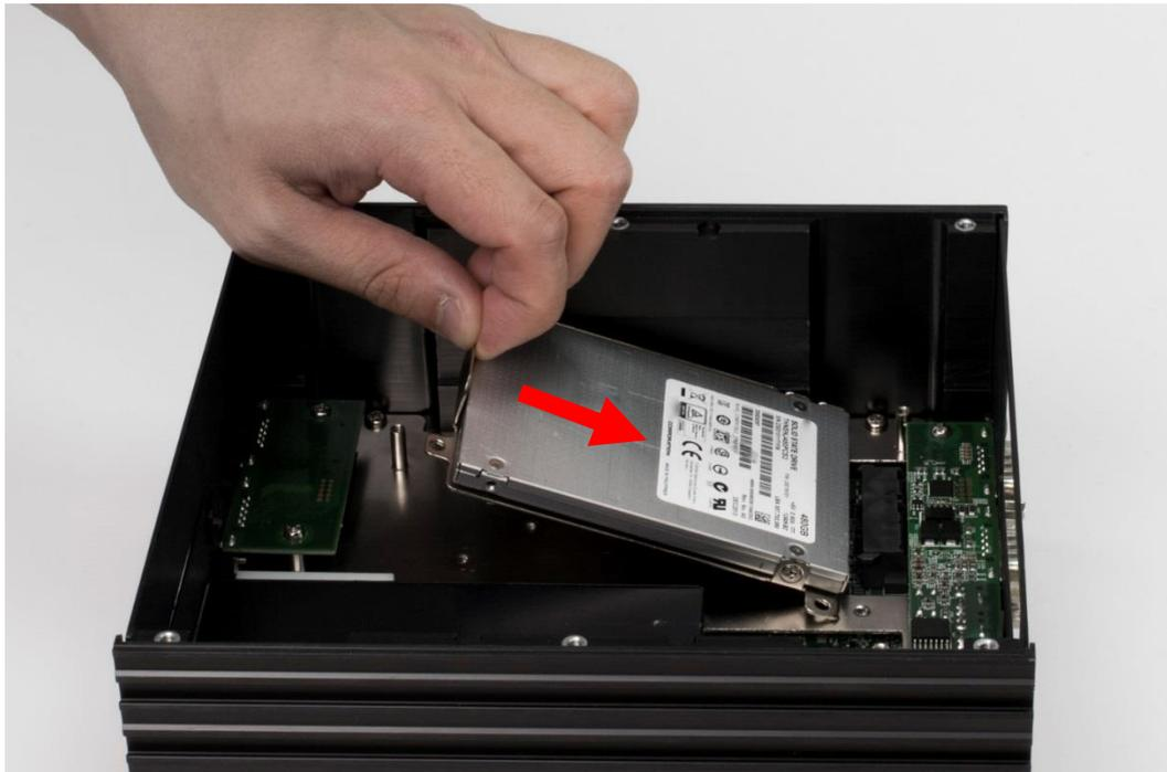
4. Fasten the three screws to lock the internal HDD bracket.
