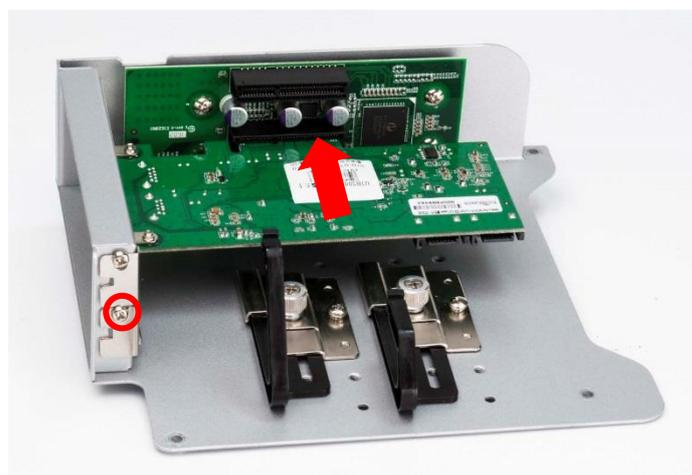
5. Adjust the arm until it holds the card firmly in place. Then fasten the sun screw on the holder.
