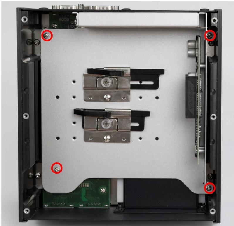
3. Now you can remove the PCIe/PCI expansion module.
