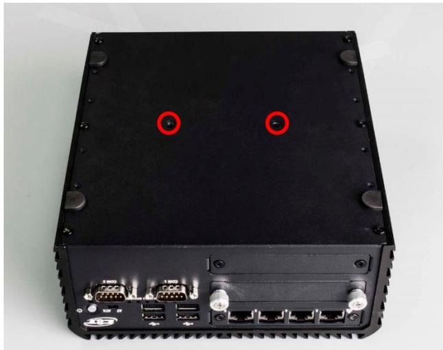
3. Place the din rail holder on top of the bottom cover and lock it with two screws (M4x5L, Nylok).
