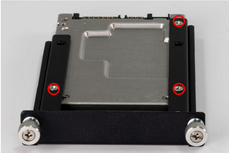
3. Slide the HDD bracket back and then fasten the sun screws.
