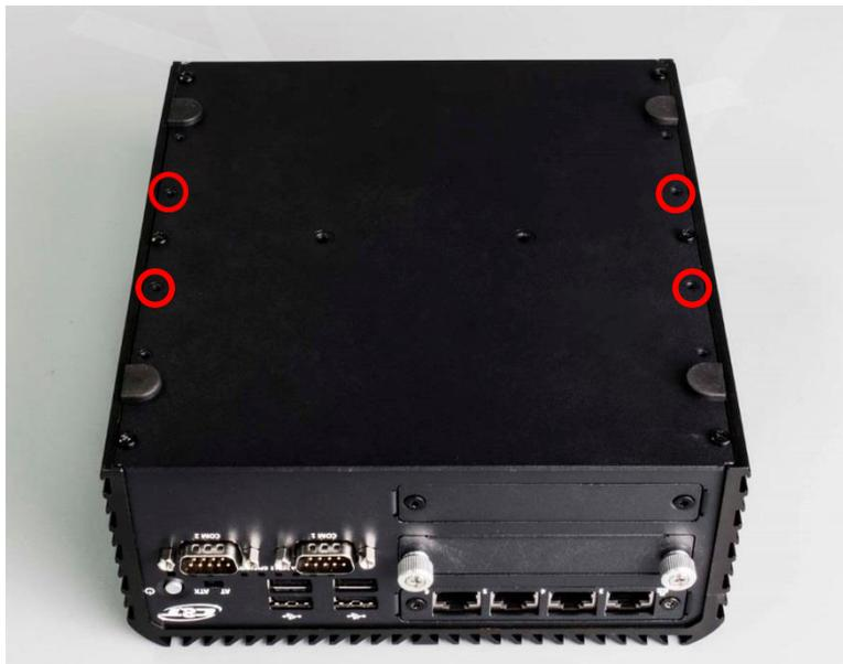
3. Lock the wall mount kit with eight screws (M3x5L, Nylok).
