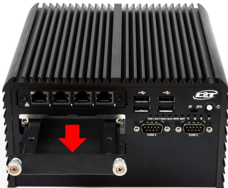
2. Lock the 2.5" HDD with HDD bracket using three screws (M3x4L).
