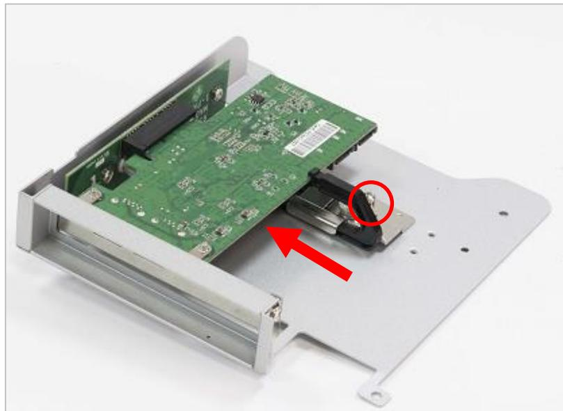
6. For RCO-3022 series, install the upper card (Card 1) first and then install the lower card (Card 2).
