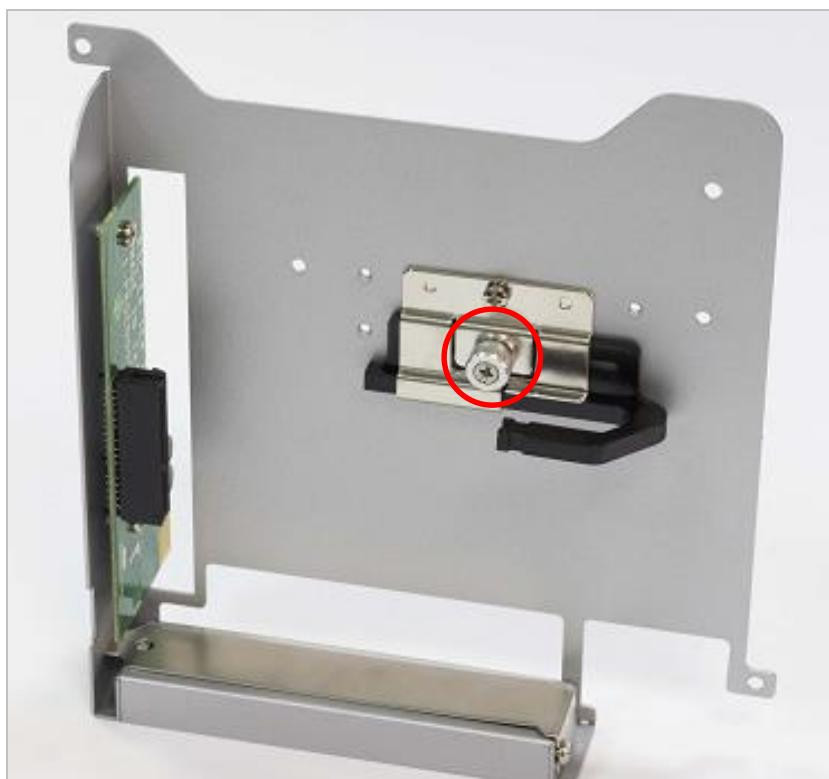
4. Install the PCIe/PCI card according to the below direction and ensure the gold finger is inserted into the slot. Then fasten the screw in the circle.
