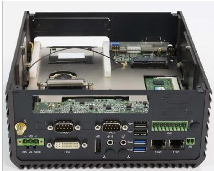
5. Assemble the antenna and antenna jack together.
