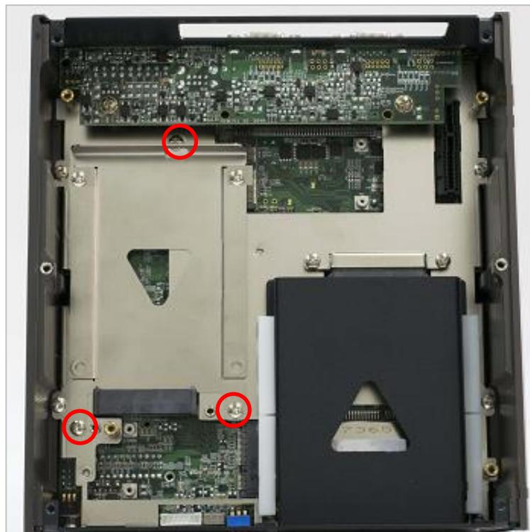
2. After removing internal SATA HDD bracket, you will be able to access the memory slot.
