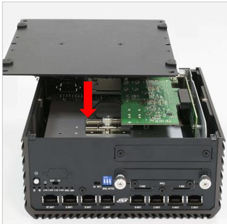
2. Lock the bottom cover with the six screws (M3x5L).
