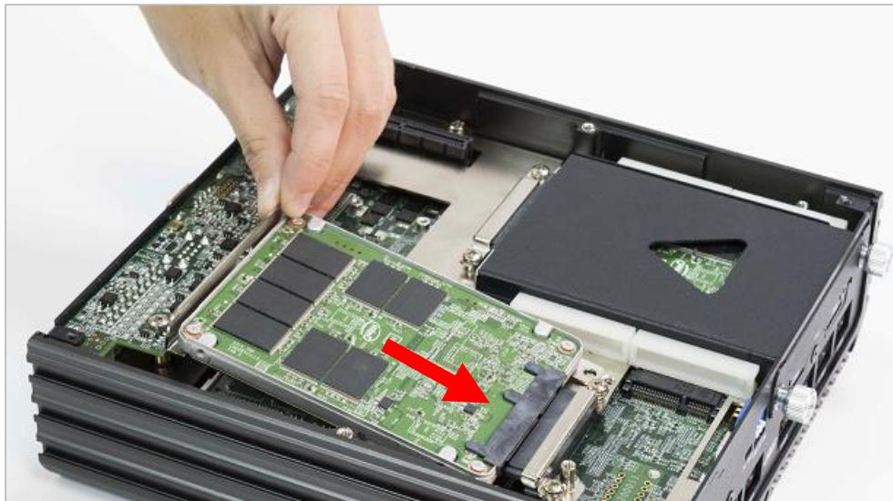
4. Fasten the three screws to lock the internal HDD bracket.
