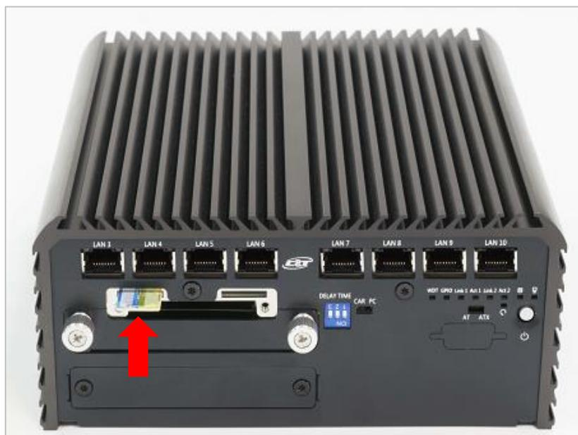
3. Please note that the installation of SIM 1 and SIM 2 has to match the installation of mini PCIe slots.
