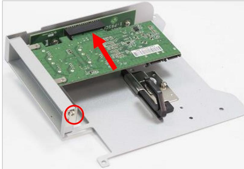
5. Adjust the arm until it holds the card firmly in place. Then fasten the sun screw on the holder.
