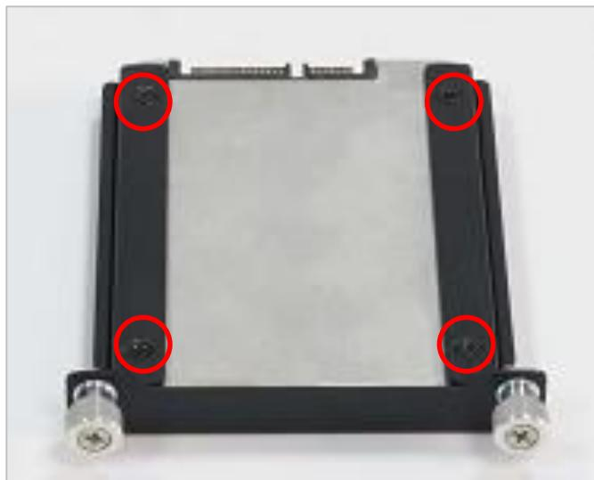
3. Slide the HDD bracket back and then fasten the sun screws.
