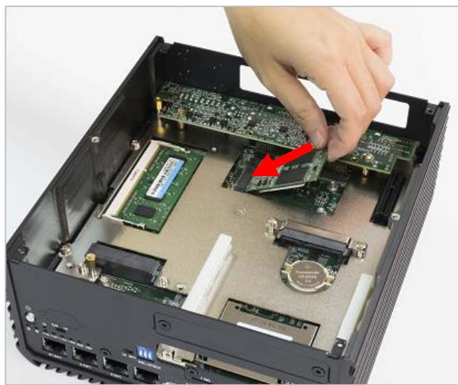
3. Press the mini PCIe card or mSATA module down and lock it with two screws (M2x3.7L).
