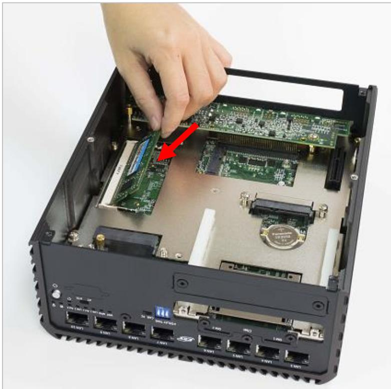
4. Press the memory module vertically downward until you hear the “click” sound. Make sure the memory module is firmly in place.
