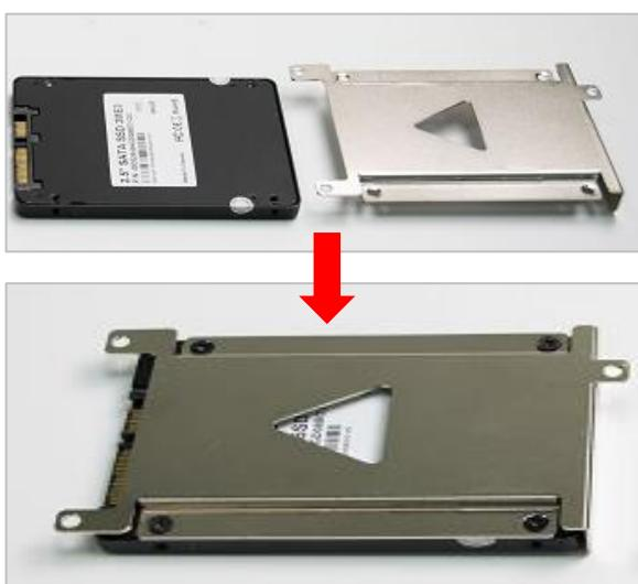
4. Install the HDD bracket following the direction below.
