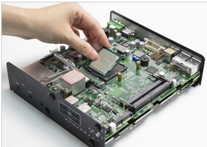
5. Press down the lever again to hold the socket cover.
