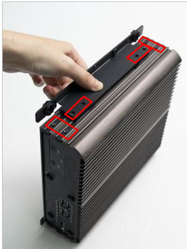
4. Lock the wall mount kit with eight screws (M3x5L, Nylok).
