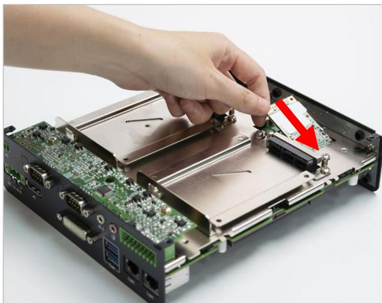
3. Press the mini PCIe card down and lock it with two screws (M2x3.7L).
