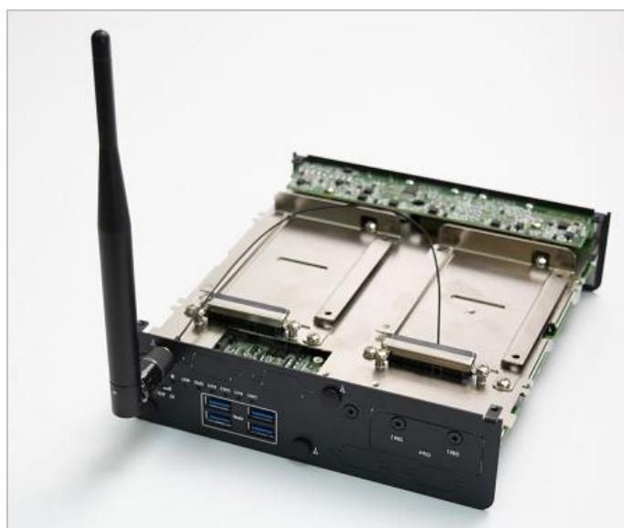
6. Attach the RF connector at the cable-end onto the communication module.
