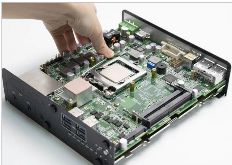
6. Paste thermal pad (1-BR0500040, 29x29x0.5mm) on the CPU.
