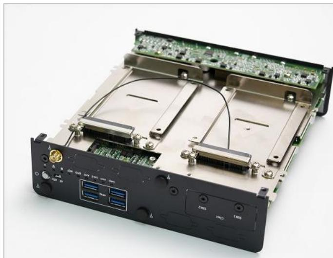
5. Assemble the antenna and antenna jack together.
