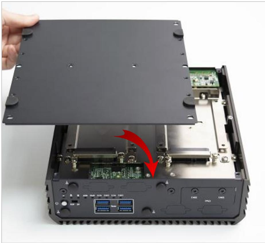
2. Lock the bottom cover with the six screws (M3x5L).
