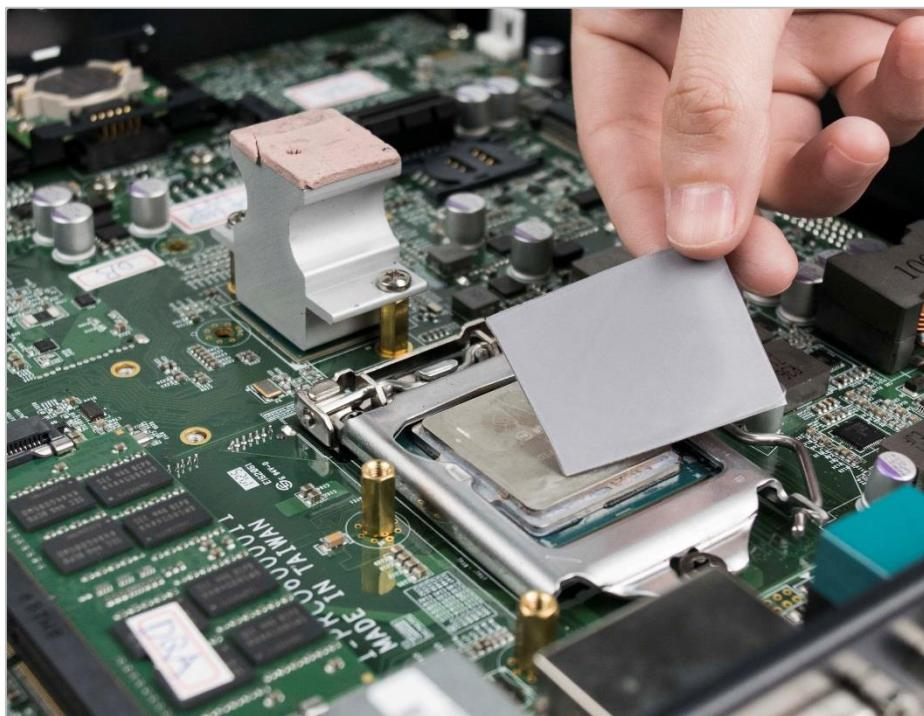
7. Place the designated heat block onto the CPU with thermal pad.
