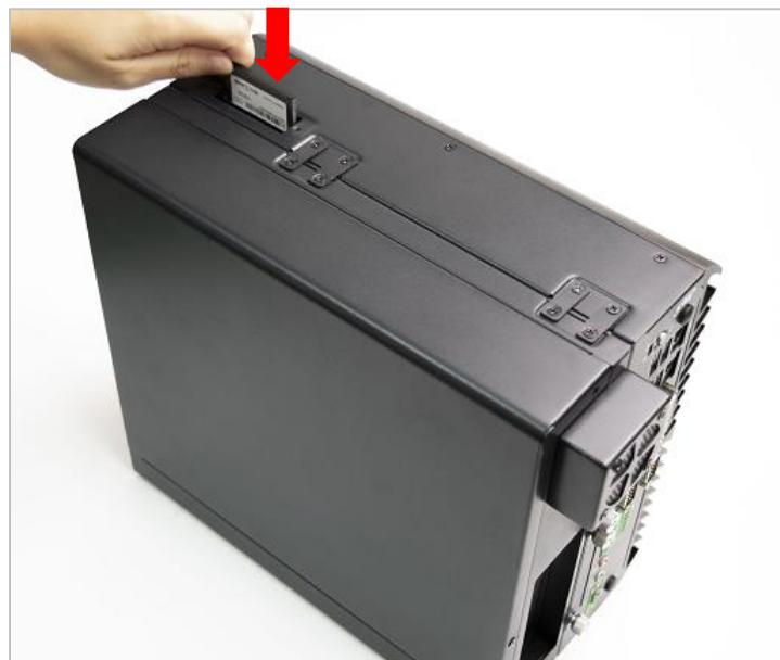
3. The socket is push-push type. Push the installed CFast card again to remove it.
