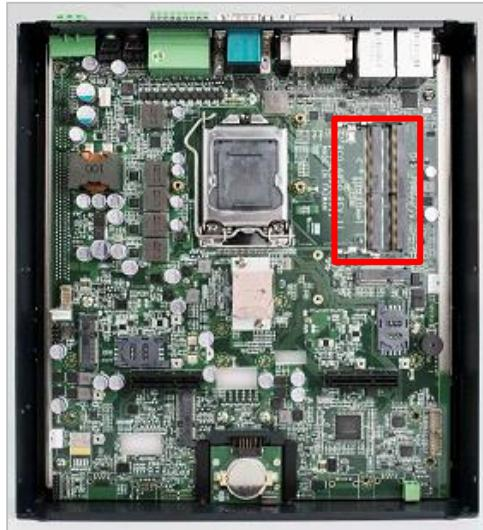
2. Insert memory module from 45 degree direction.
