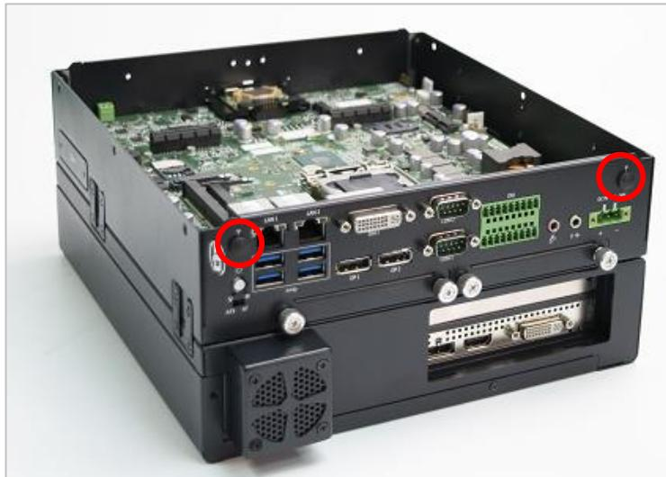
2. Remove antenna hole cover on the front panel.
