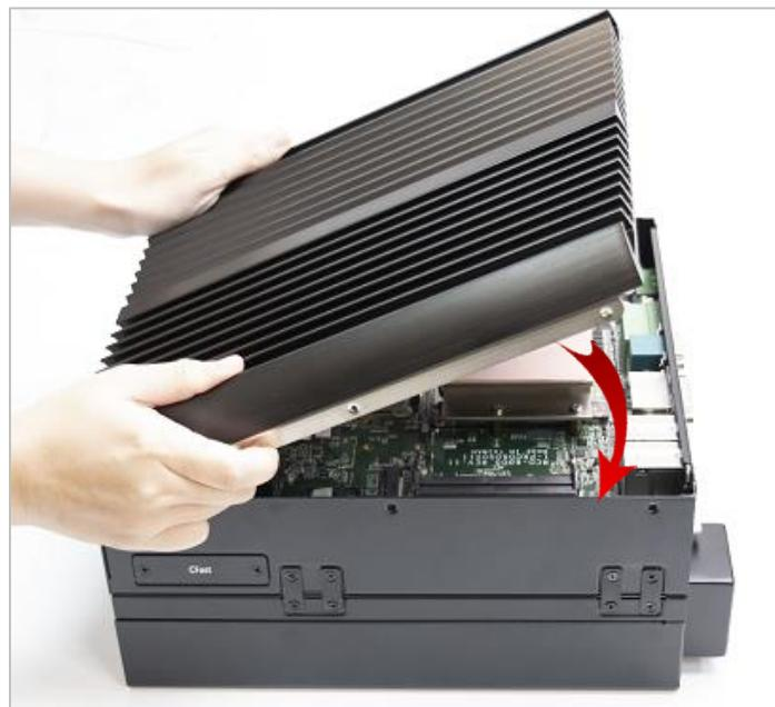
3. Fasten the six screws on the system top side and bottom side.
