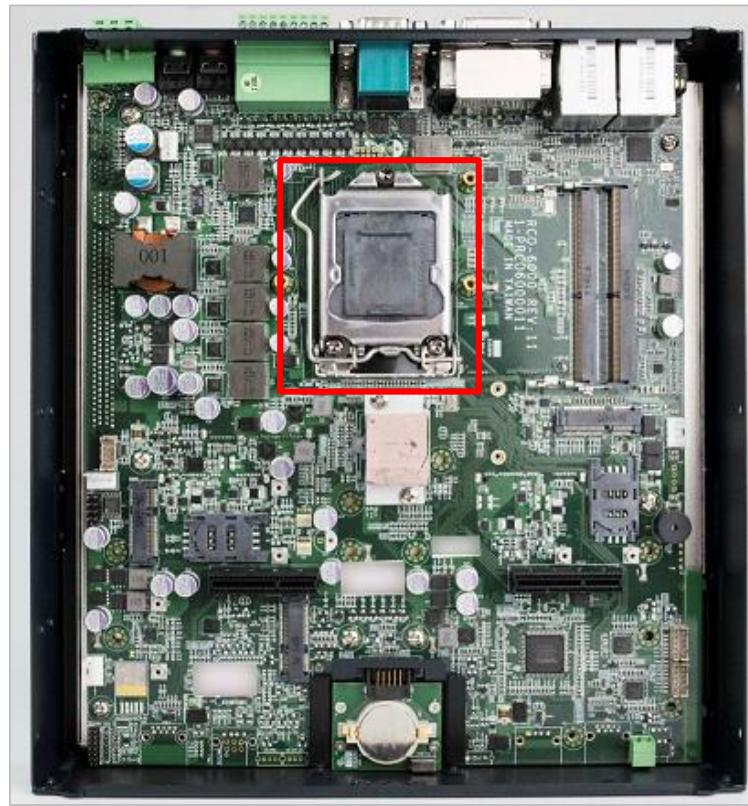
2. Press down the CPU socket lever in order to open the socket cover.
