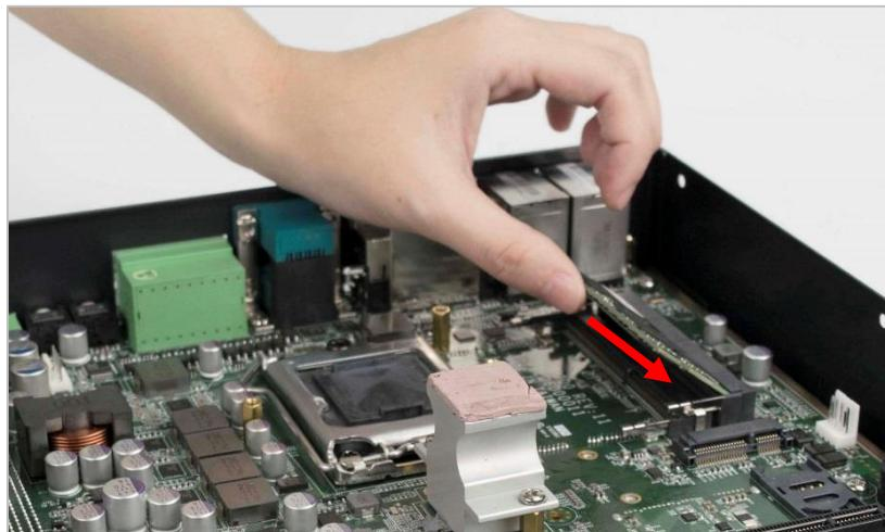
3. Press the memory module vertically downward until you hear the “click” sound. Make sure the memory module is firmly in place.
