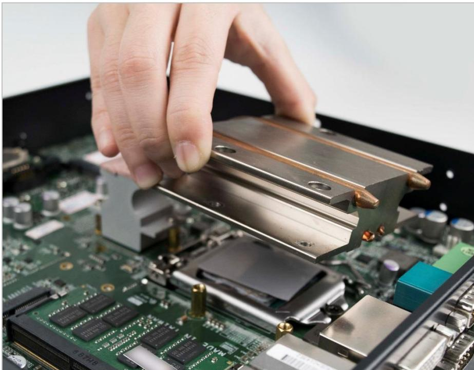
8. Lock the heat block with three screws. Screw driver will able to penetrate through the holes on the top in order to fasten the screws with copper stud.
