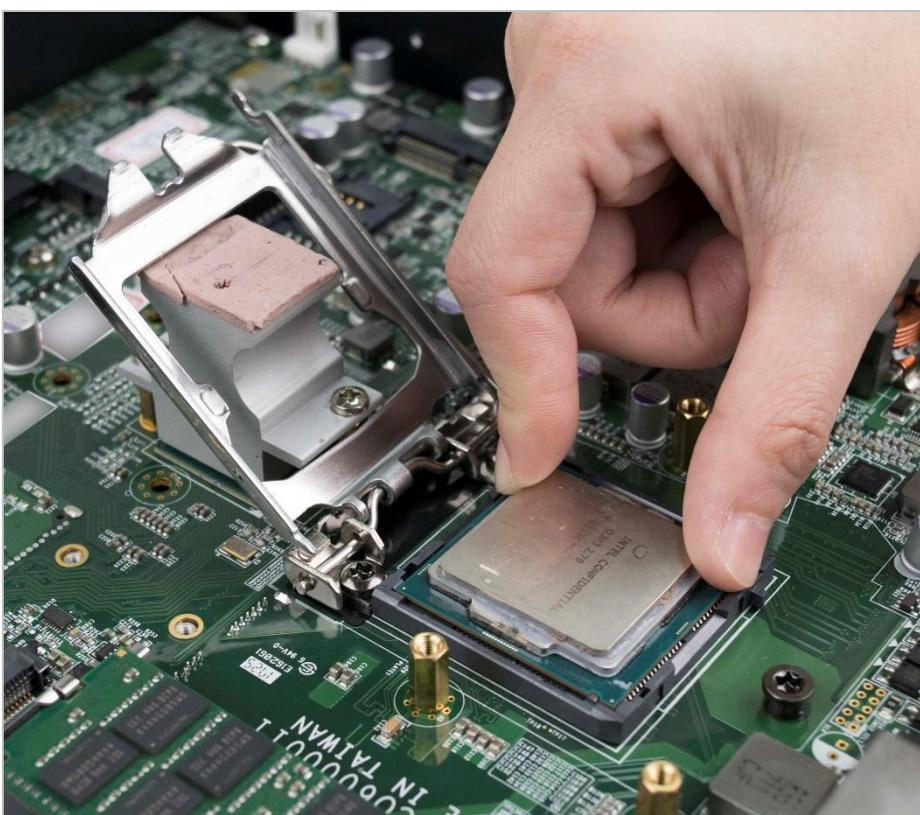
5. Press down the lever again to hold the socket cover.
