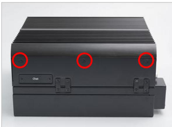
2. Unscrew the 3 screws on the bottom side.
