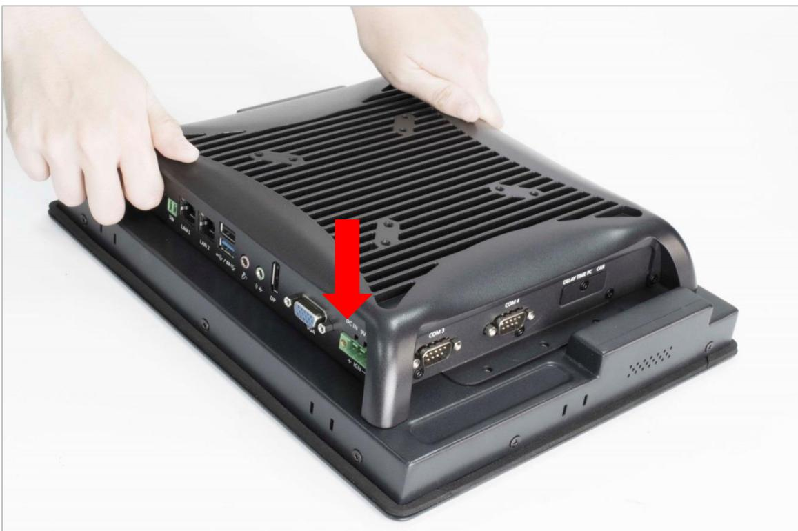
3. Lock the below 6 screws (M4X5L) to finish assembly.
