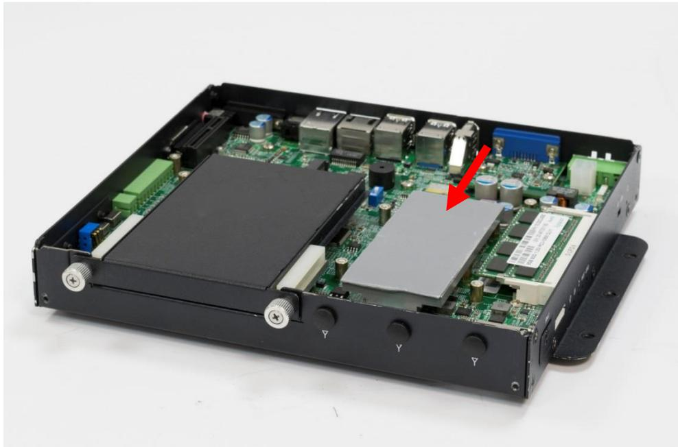
2. Close the chassis top cover following the below direction and make sure the aluminum part on the top cover is touching the thermal pad on CPU thermal block.
