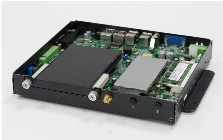
5. Attach the RF connector at the cable-end onto the communication module.
