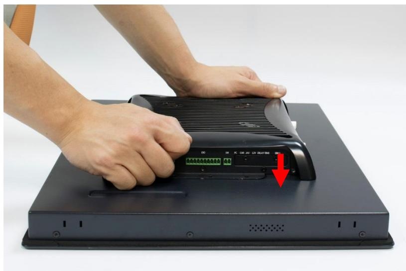
3. Lock the below 6 screws (M4x5L).
