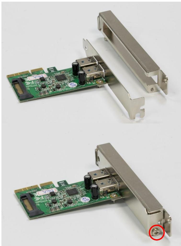
4. Install the PCIe/PCI card according to the below direction and then push the card towards the slot to ensure the gold finger is firmly inserted into the slot.
