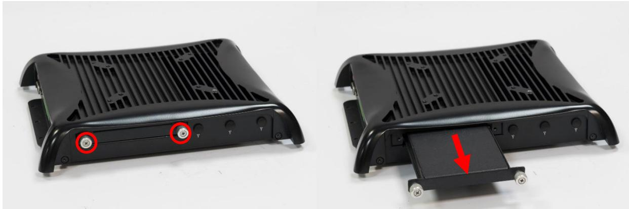
3. Lock the 2.5" HDD with HDD bracket using four screws (M3x4L).
