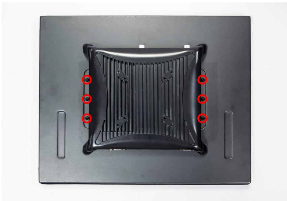
2. Lift up the PC module to separate it from the display module.
