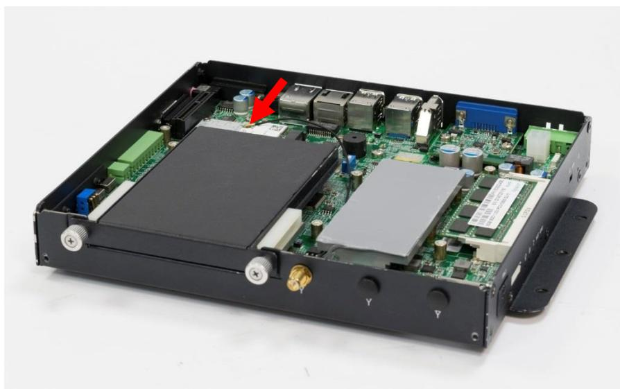
6. Assemble the antenna and antenna jack together.
