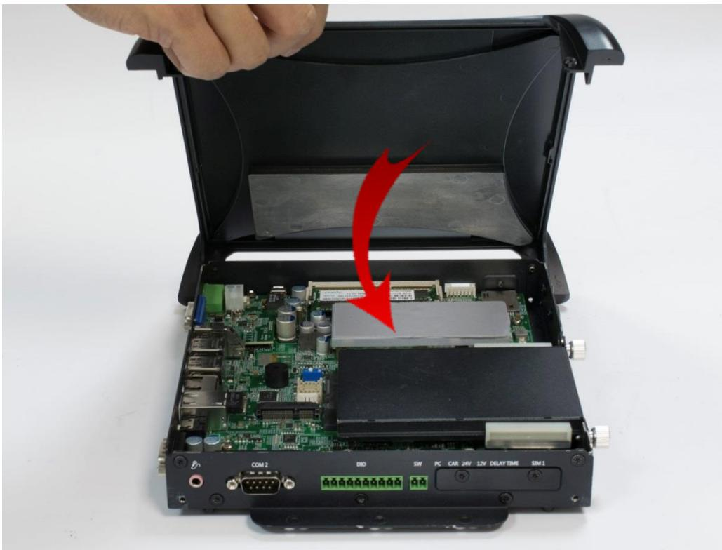
3. Fasten the six screws (M3x5L) to lock the system body with top cover.
