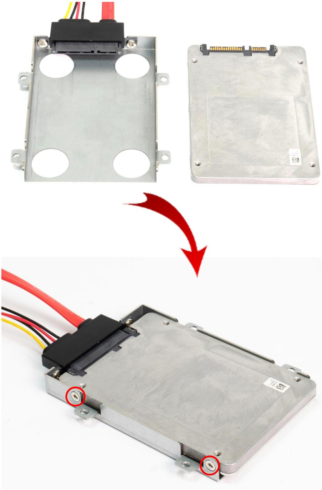
2. Fasten the four screws (M3x5L) to lock the HDD bracket in place.
