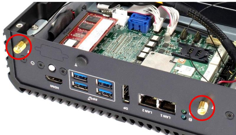
3. Put on washer and fasten the nut with antenna jack.
