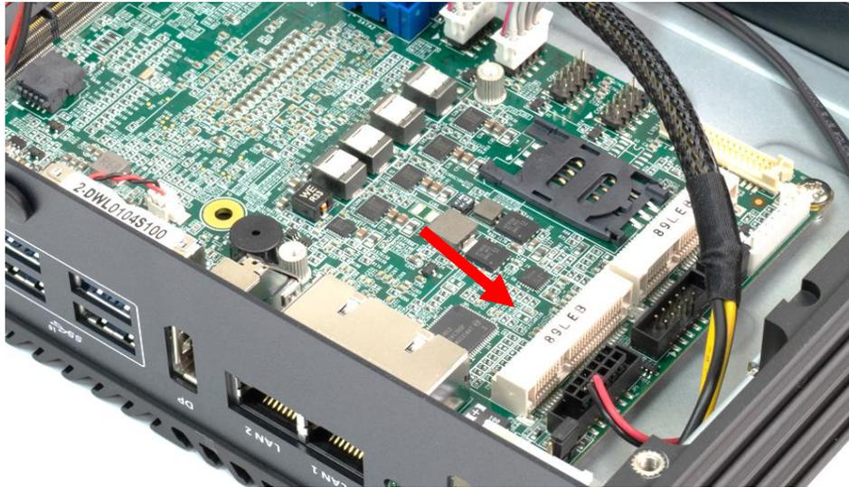
2. Insert mini PCIe card or mSATA module from 45 degree direction.
