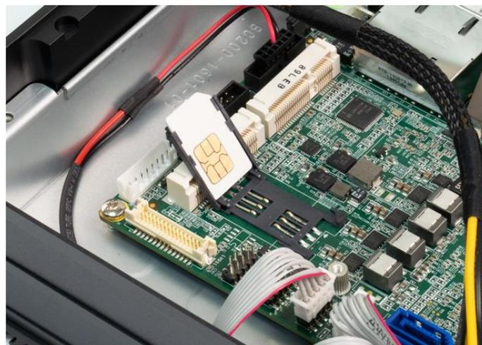
3. Following the below direction until you hear the “click” sound. Make sure the SIM card is firmly in place.
