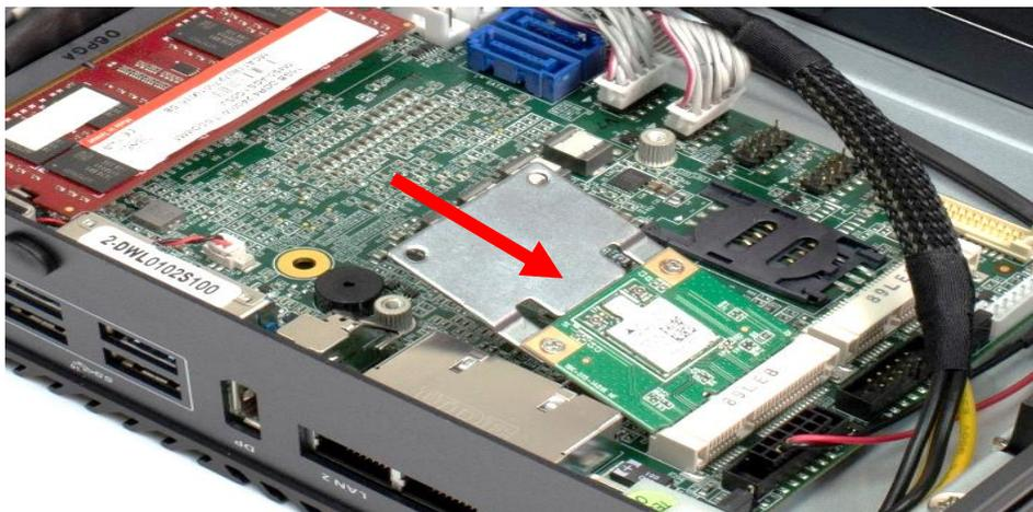
3. Press the mini PCIe card or mSATA module down and lock it with one screws (M2.5x3.7L).
