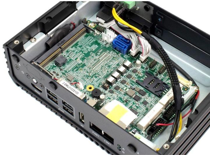
2. Insert memory module from 45 degree direction.
